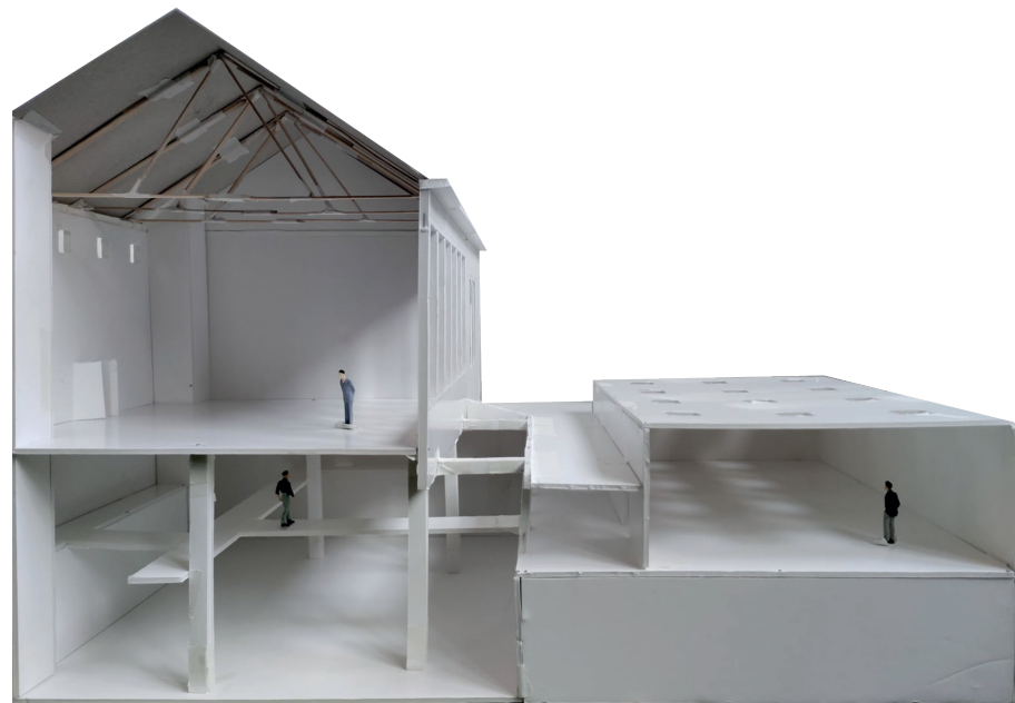
Figure 90. The basement originally had skylight in the roof. At a certain period a new construction was added on top of it that poured concrete in the former skylights. The dark basement can be activated by opening up the roof with skylights to make the space underneath more qualitative with natural daylight
