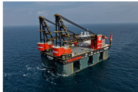
(b) Semi-submersible Crane Vessel ["Heerema Sign with Sembcorp for Sofia OWF HVDC Offshore Converter Platform", 2021]
