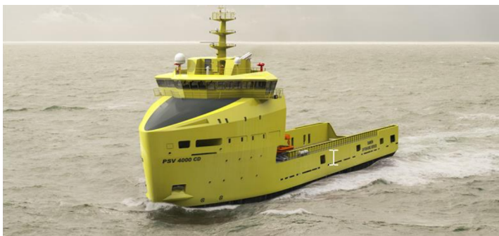
Figure 3.1: A 3D rendering of the PSV 4000 CD [“The complete Platform Supply Vessel”, n.d.]
