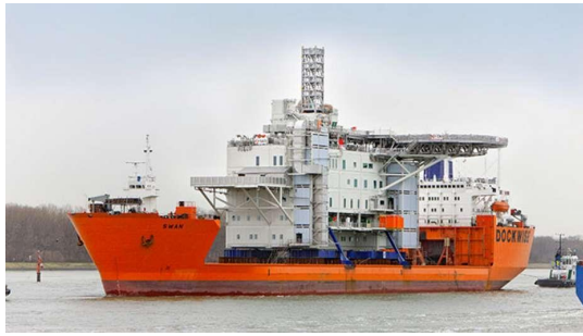
(a) The 'Swan' semi-submersible transport vessel [HeavyLiftPFI, 2021]
