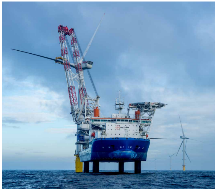
Figure 3.4: Image of the 'Vole au vent' lifting itself out of the water ["Vole au vent: Offshore Jack-Up installation vessel", n.d.]
