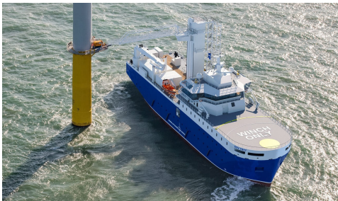
(a) Walk to Work Vessel ["Damen SOV 7017/ SOV 8417 Walk to Work Vessel", n.d.]
