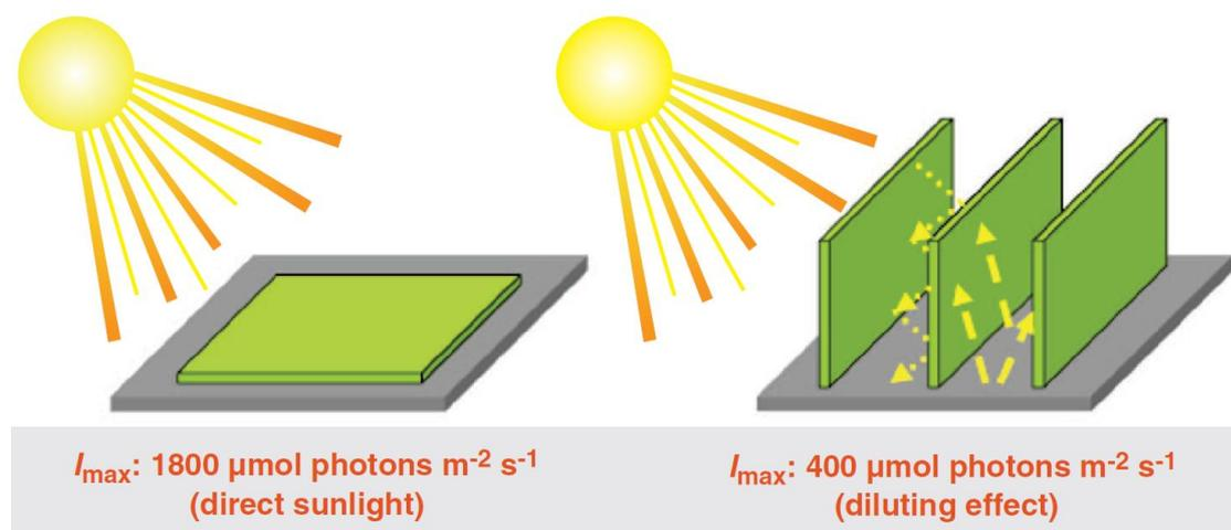
Figure 19: horizontal versus vertical flat panel photobioreactor (Wijffels & Barbosa, 2010, p. 796)
