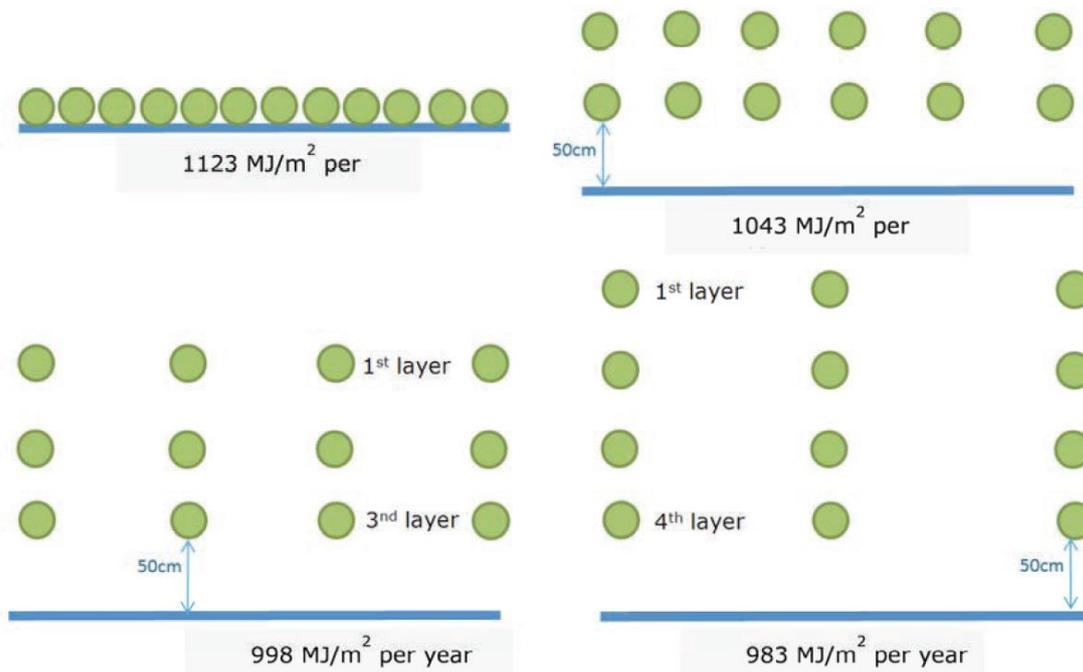
Figure 43: same amount of bioreactor tubes with different configurations and solar capture (Hemming et al., 2012, p. 63)
