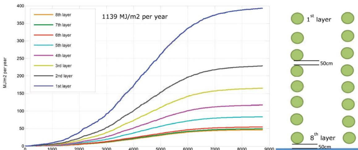
Figure 44: light absorption per layer with a vertical system with a vertical cavity of 50 cm and tube diameter of 110 mm (Hemming et al., 2012, p. 64)
