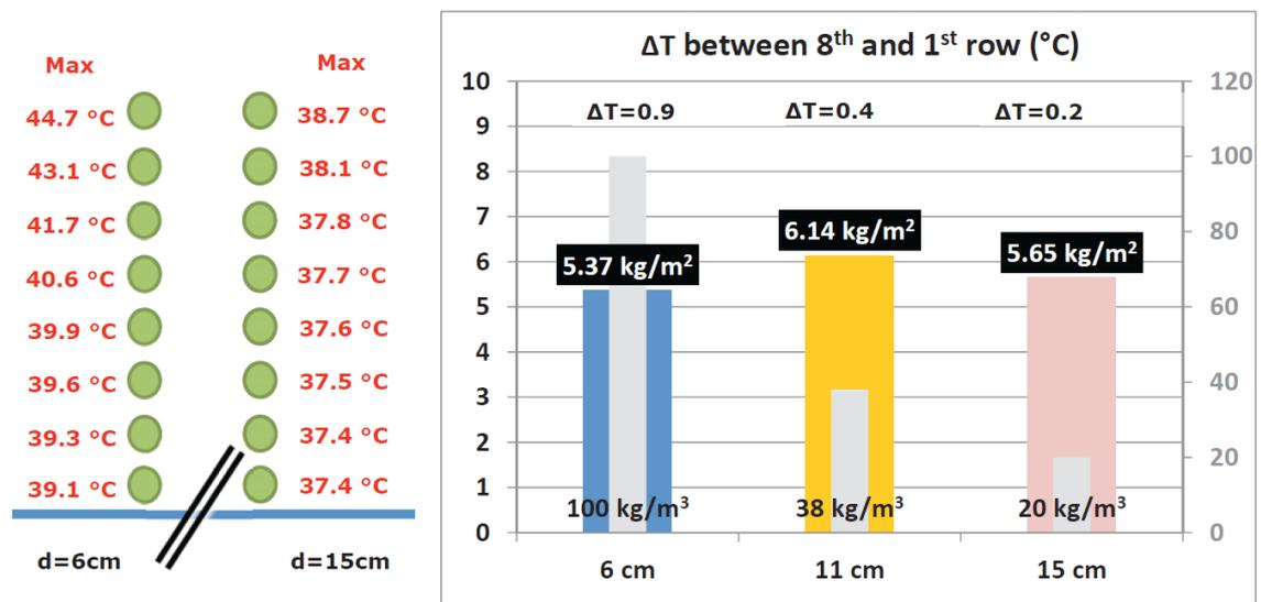
Figure 48: temperatures and productivity with 8 stacked photobioreactors (Hemming et al., 2012, p. 70)
