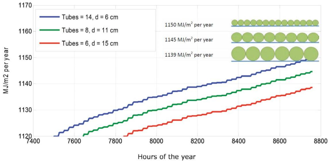
Figure 41: light capture of bioreactor tubes with different diameters and the same ground surface and different volumes (Hemming et al., 2012, p. 61)
