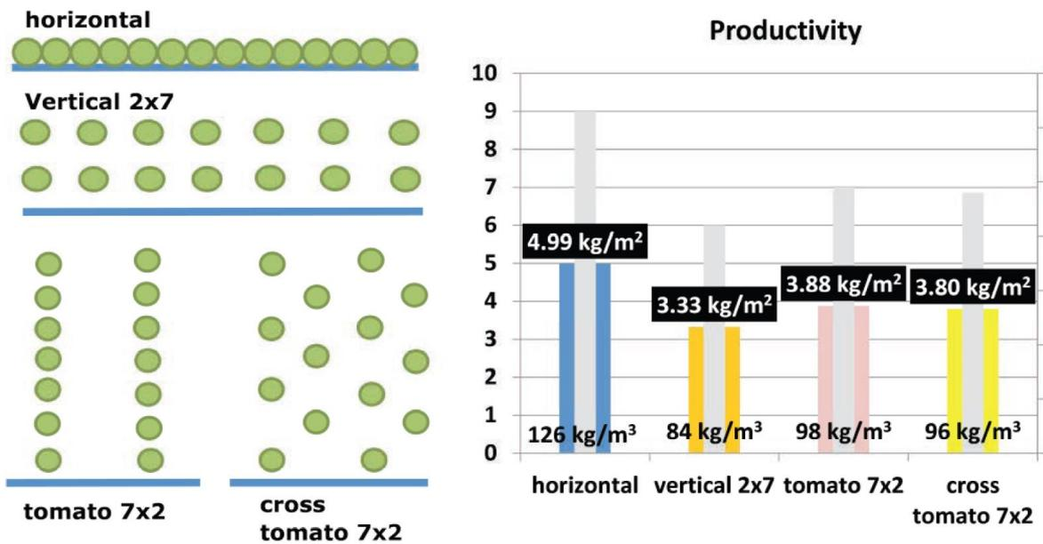
Figure 49: different setups for photobioreactor tubes (Hemming et al., 2012, p. 76)
