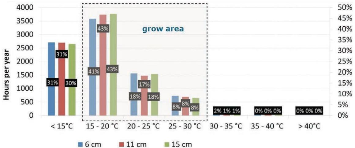
Figure 47: measured temperatures of one year in a two layered photobioreactor (Hemming et al., 2012, p. 68)
