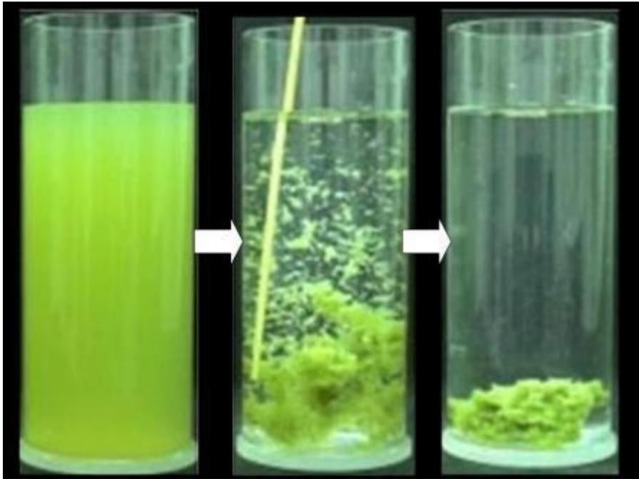
Figuur 55: flocculation process (Zhiting, 2011)
