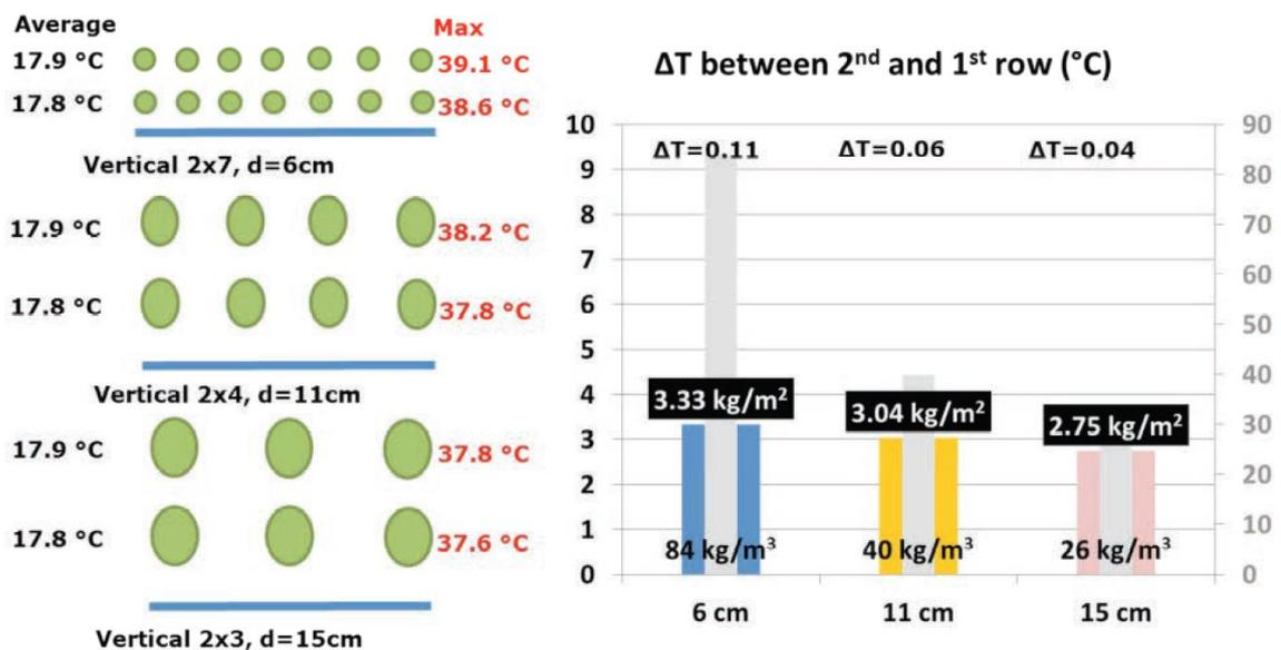
Figure 46: temperature difference with variable diameter (Hemming et al., 2012, p. 67)
