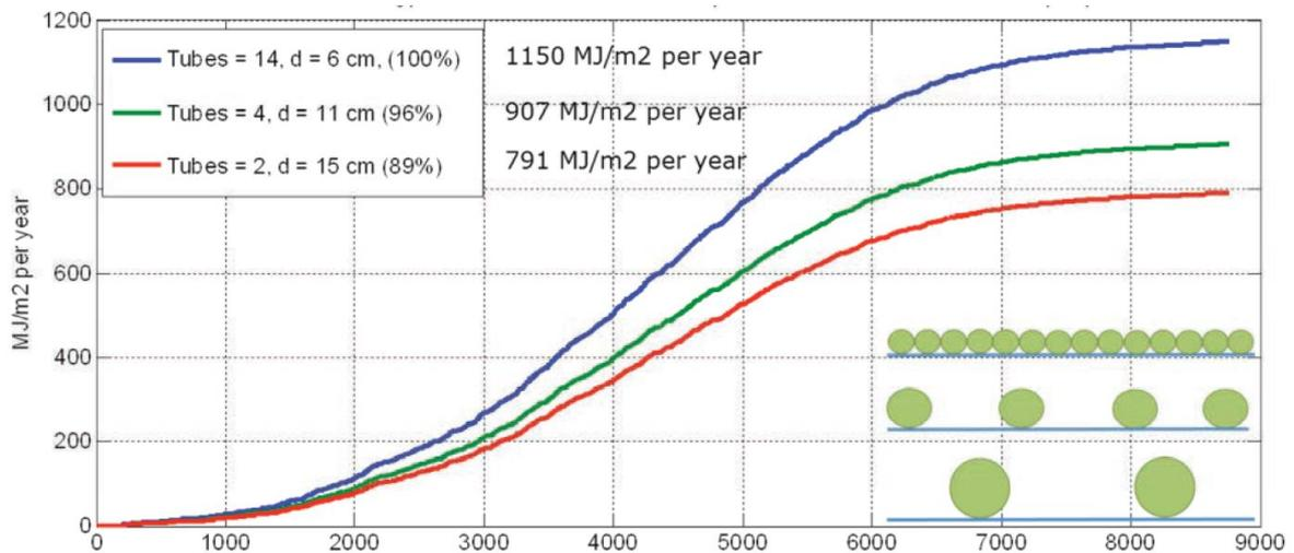
Figure 42: light capture of bioreactor tubes with different diameters and the same ground surface with the same volumes (Hemming et al., 2012, p. 62)
