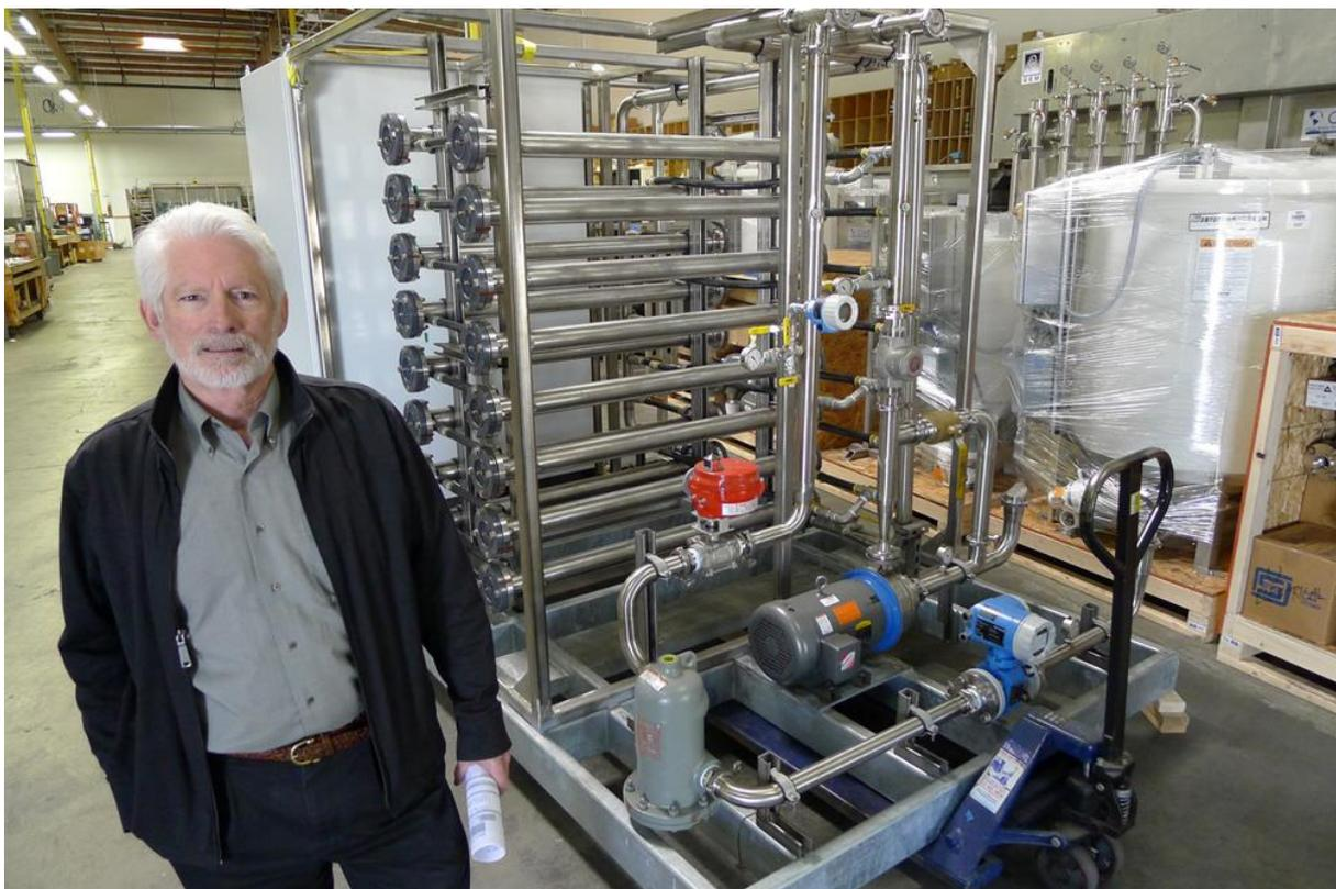
Figure 54: Single Step Extraction machine (Originoil, 2012)
