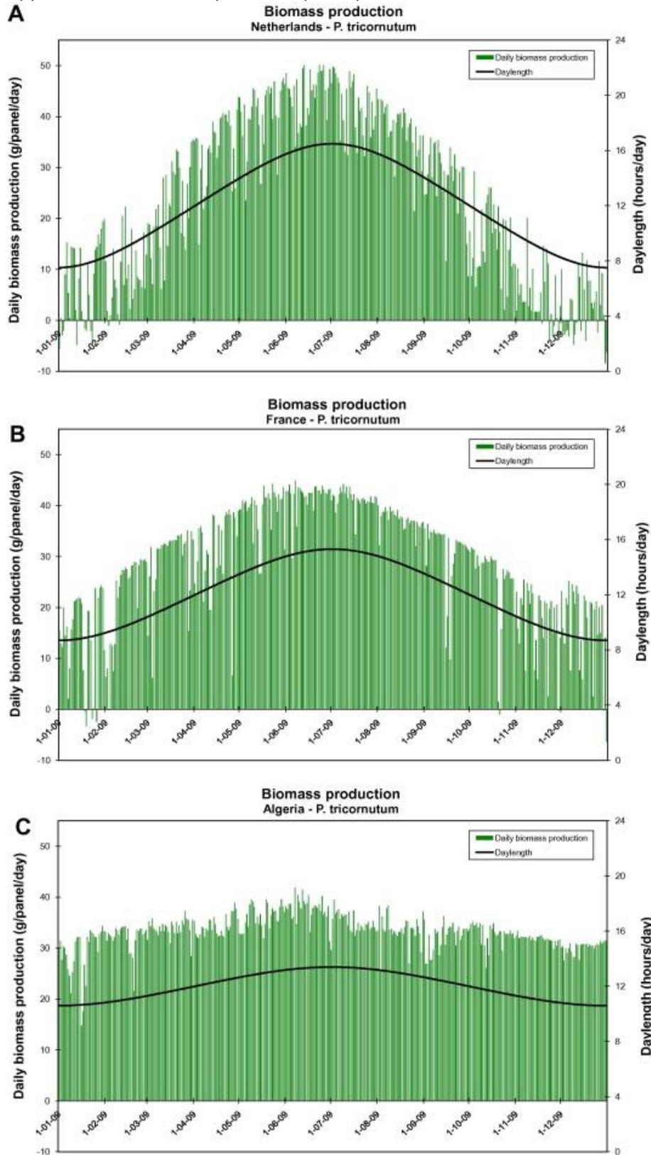
Figure 52: daily biomass production on three locations with flat panel photo bioreactors (Slegers et al., 2010, p. 3345)
