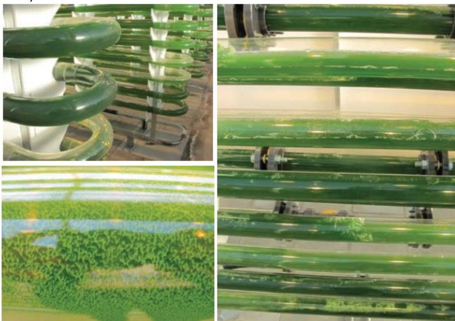
Figure 18: microalgae growing on the inner surface of the tubes (Hemming et al., 2012)
