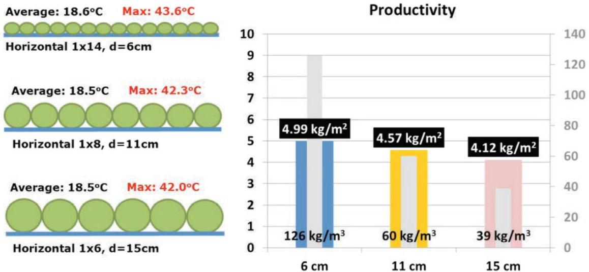
Figure 45: temperature difference with variable diameter (Hemming et al., 2012, p. 66)
