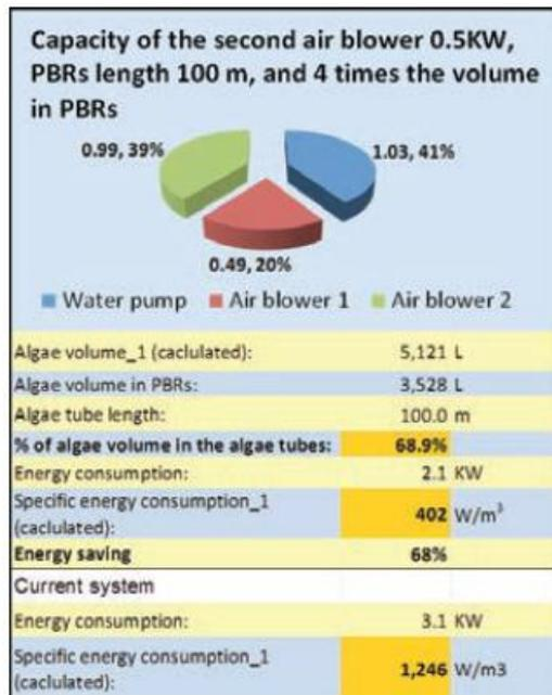
Figure 51: test system with basic optimization (Hemming et al., 2012)
