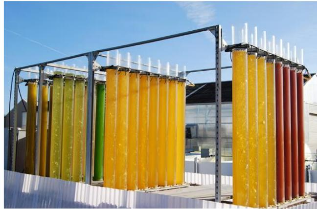
Figure 4: tubular photobioreactors (Schwartz, 2012)
