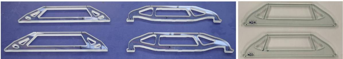
**Fig. 16** Images of fabricated waterjet cut float glass beam specimen. The volume-based is on left, the stress-based is in middle, and in a separate photo the stiffness-based is on right
