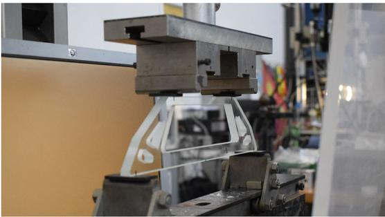
**Fig. 18** Testing setup for 4-point bending load case on fabricated glass beams. The loading apparatus and supports (with neoprene pads) are shown. The screen behind the testing sample is used for the cross-polarization process. In this case, a volume-based design without tape is placed in the testing machine
