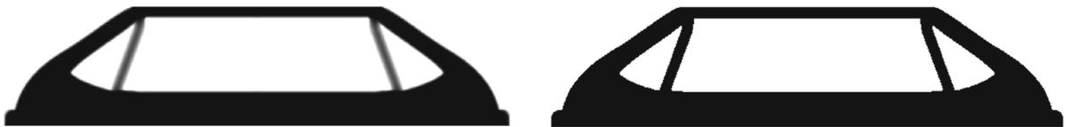
**Fig. 15** On left, the geometry output by the optimization, while right shows the results after rounding is used to eliminate grey elements
