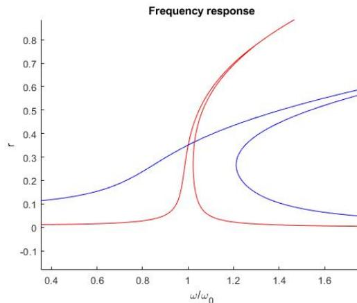
Figure 5.8: The blue line ( $\beta = 0.1$ ) shows less unstable solutions compared to the red one ( $\beta = 1$ ).
