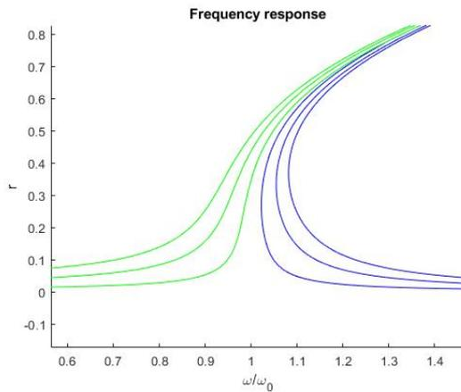
Figure 5.5: Hardening quintic Duffing oscillator, vaying damping coefficient.
