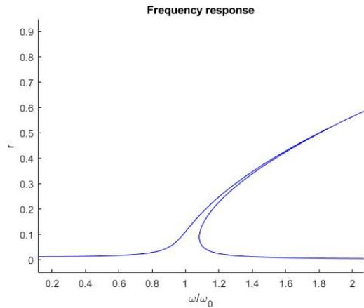
Figure 5.10: Hardening system,  $\alpha, \psi > 0$ .
