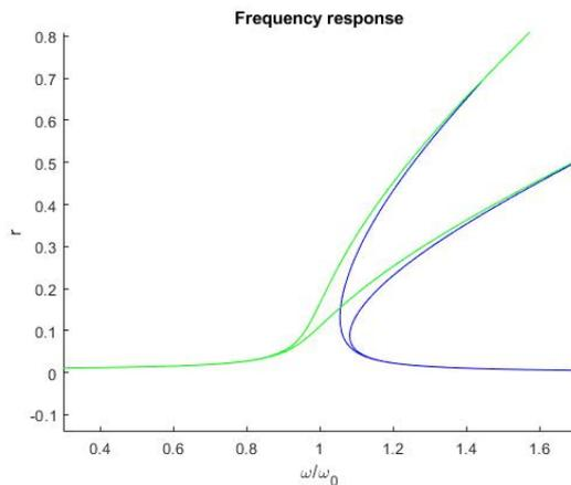
Figure 5.3: Hardening cubic Duffing oscillator.
