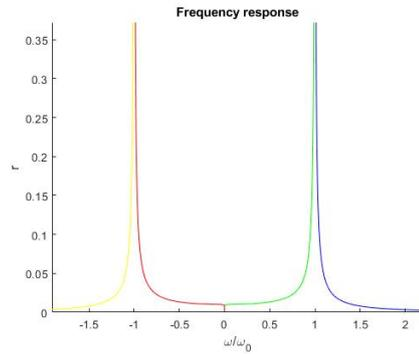
Figure 5.1: Amplitude-phase relation, values of  $\alpha = 0, \psi = 0, \beta = 1, \delta = 0.01, \gamma = 0.01$ .
