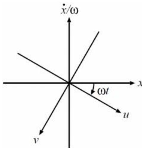
Figure 4.1: Van der Pol transformation in a 2-D plane[2].
