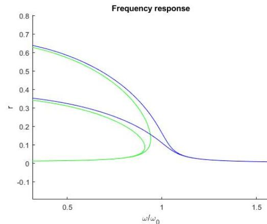
Figure 5.4: Softening cubic Duffing oscillator.
