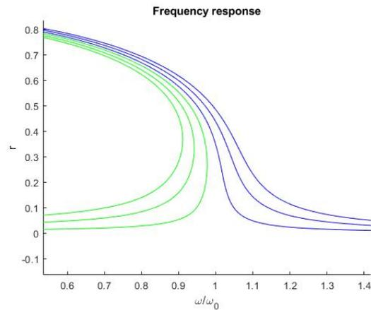
Figure 5.6: Softening quintic Duffing oscillator, vaying damping coefficient.
