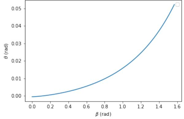
**Figure 2.** The pitch setting is dictated by  $\beta$ , which depends on the height and distance between the MAV and target (Figure 1).
