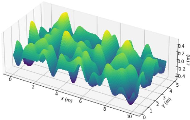
**Figure 15.** Perlin noise adds a realistic terrain profile to a ground surface. By training on such ground surface, a robust controller is evolved.
