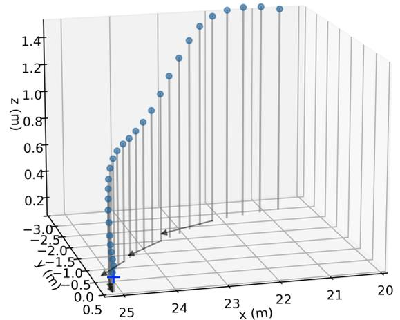
**Figure 11.** The dots indicate the position of the MAV, which is sampled every second. For more clarity, a bar is added that displays the position at ground surface level. A  $0.25rad$  offset is introduced in the heading signal, which causes the MAV to approach the target with a slight curve.
