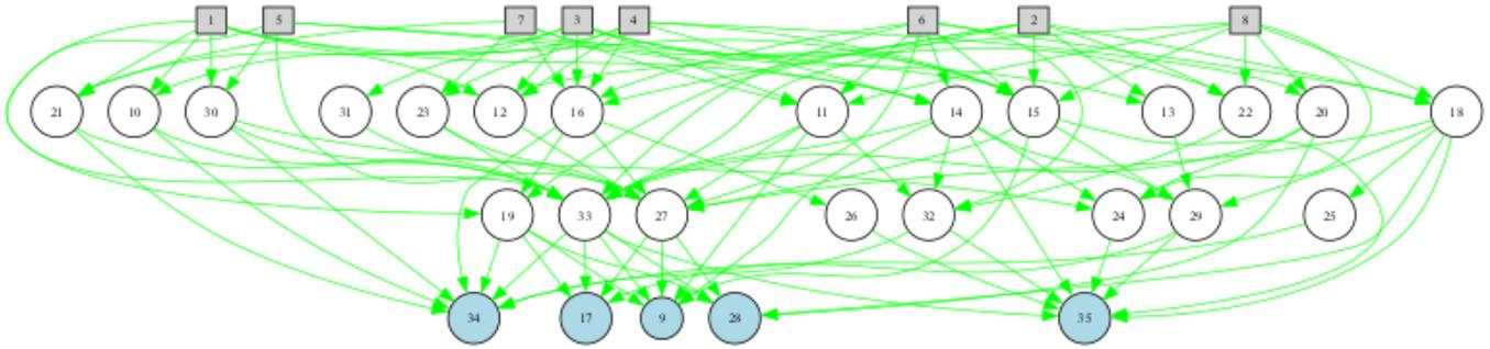
**Figure 14.** An evolved network using the NEAT-SNN module. The square nodes in the top layer represent the input neurons while the blue shaded neurons on the bottom are the output neurons. The remaining neurons are part of the hidden layers. It should be noted that the networks starts learning without any direction connection between the input and output layer. This means that every input signal travels through a neuron before reaching the output neurons.
