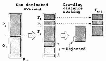
**Figure 7.1:** The figure is adapted from [84] showing the NSGA-II selection procedure.
