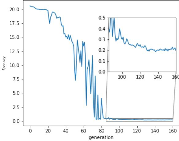
Figure 5. The learning curve shows objective evaluations of the best scoring individual every generation. The highlighted area shows that the controller has converged, which means that the MAV reaches the end of the simulation environment. When reaching the end, the only penalty given is due to a difference for  $u$  and  $\psi$  between the actual and setpoint
