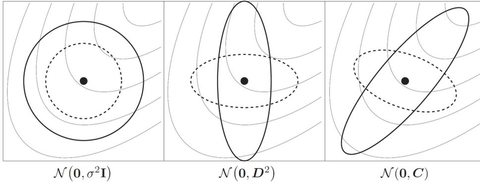
**Figure 7.5:** Figure shows the different sampling distributions in the CMA-ES algorithm.  $C$  is the positive definite full covariance matrix. Adapted from [93]
