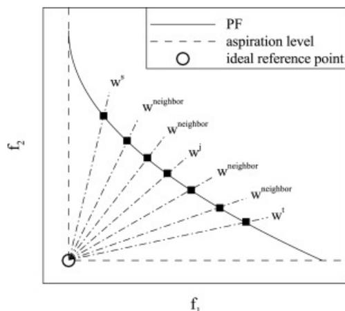
**Figure 7.4:** The figure is adapted from [89] showing the ideal pathway of solution on the Pareto front to follow.
