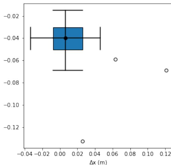
**Figure 13. A 2D box plot of the touch-down locations of 100 executed landings.**
