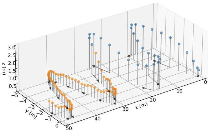
**Figure 10.** During cruise, a sine wave ground path is followed. The dots indicate the MAV's position and are sampled every second. Due to a lower pitch and consequently forward speed, the dots are closer to each other in the second part of the trajectory.
