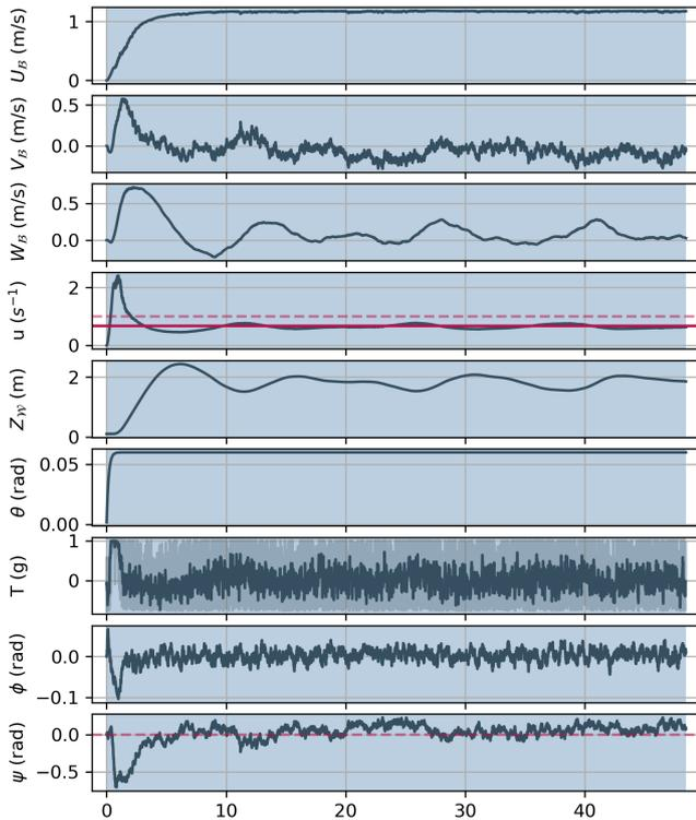
**Figure 7. Body speeds  $U_C$ ,  $V_C$ ,  $W_C$ , ventral flow  $u$ , height, pitch, thrust, heading and roll for a simulated take-off. The dashed red lines indicate the set point of variables  $u$  and  $\psi$  during learning. The continuous red line shows the controller's actual set point for  $u$ . Since the thrust signal  $T$  is very noisy, an overlay is plotted that averages the last 10 time steps of  $T$ .**
