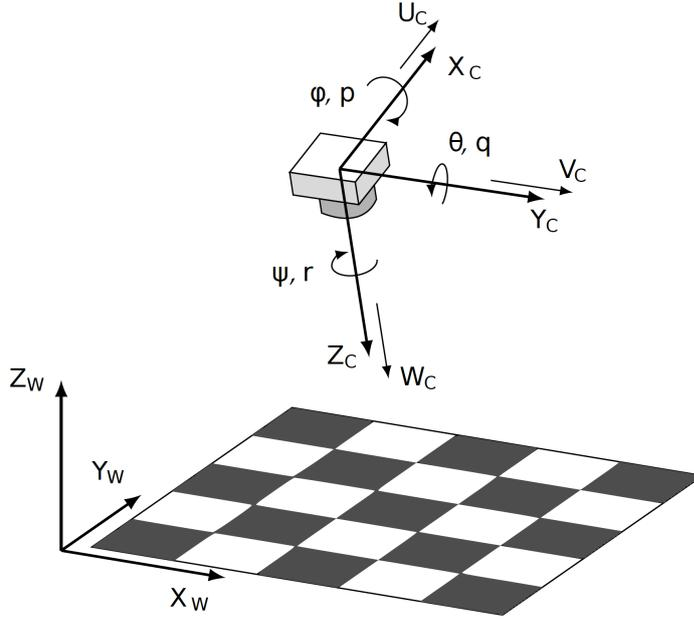
**Figure 5.1:** Adopted from [39]. Two reference frames are present, namely of the world  $W$  and camera  $C$ . The motion of the camera  $C$  is described by the translational velocities  $(U, V, W)$ , the Euler angles  $(\phi, \theta, \psi)$  and rotational rates  $(p, q, r)$ .
