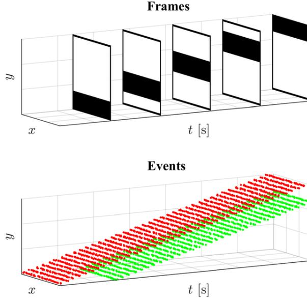
**Figure 5.2:** Illustration of the observed difference between frame and event based camera's. As the black bar in the image moves up, event-based camera's only respond to the leading and trailing edge of the black surface, since brightness changes are observed here. The green and red colours represent polarity of a positive and negative change, respectively.
