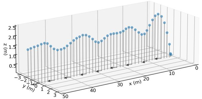
**Figure 8. The dots indicate the position of the MAV, which is sampled every second. For more clarity, a bar is added that displays the position at ground surface level. The arrows indicate the direction of travel.**
