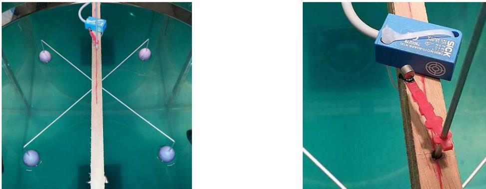
**Figure 5** Left: floating quadripod to determine flow circulation consisting of four egg shaped hollow balls connected to a 0.30 m cross shaped frame of 3 mm diameter aluminium rods. Right: magnetic device recording the quadripod revolution rate.
