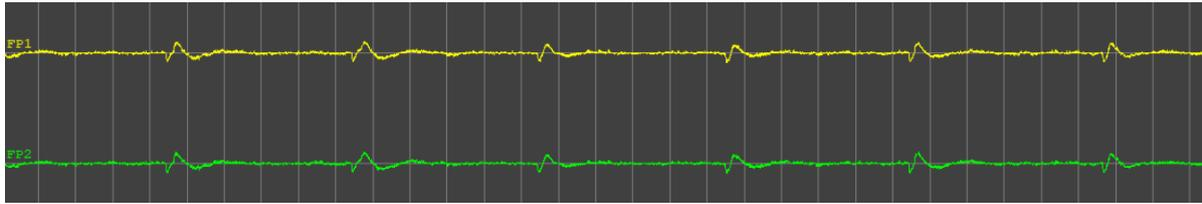
**Figure 6.4:** Measured raw data signal from FP1 and FP2 during several blink events
