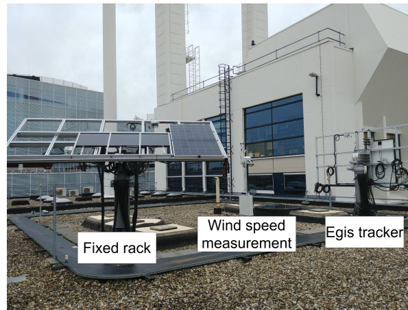
Figure 1.3: Current outdoor PV measurement setup at the TU Delft [1]
