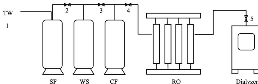
**Fig. 1** Process flow diagram. (TW-tap water, SF-sand filtration, WS-water softening, CF-carbon filtration, RO-reverse osmosis; 1-5 means the sampling port).
