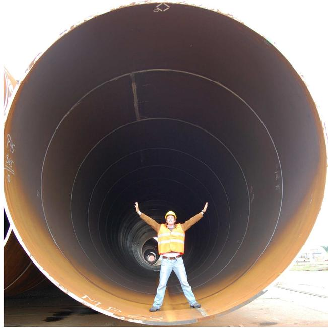
**Figure 1.4:** The author standing inside a monopile which is ready to be shipped out and installed at Sheringham Shoal wind farm. The cross section of this particular monopile has a diameter of 5.5m and a wall thickness of 6.5cm.
