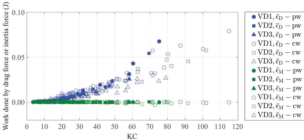
Fig. 6. The relation between  $KC$  number and the work done by drag force ( $\bar{\epsilon}_D$ ) or inertia force ( $\bar{\epsilon}_M$ ) over a wave period. ‘pw’ stands for wave-only conditions and ‘cw’ stands for current wave conditions.
