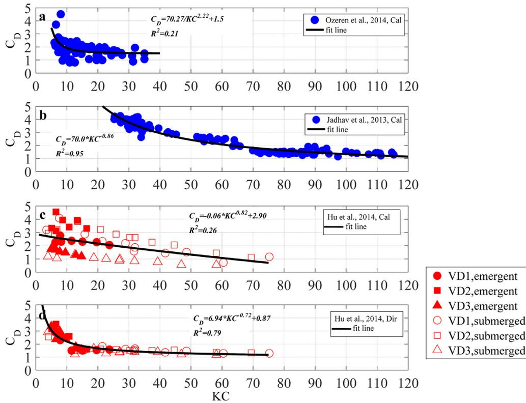
Fig. 7. Relation between  $KC$  and  $C_D$  based on various data source. (a) is based on calibrated  $C_D$  in Ozeren et al. (2014); (b) is based on calibrated  $C_D$  in Jadhav et al. (2013); (c) is based on calibrated  $C_D$  in Hu et al. (2014); (d) is based on  $C_D$  data that are derived by the direct measurement method in Hu et al. (2014).
