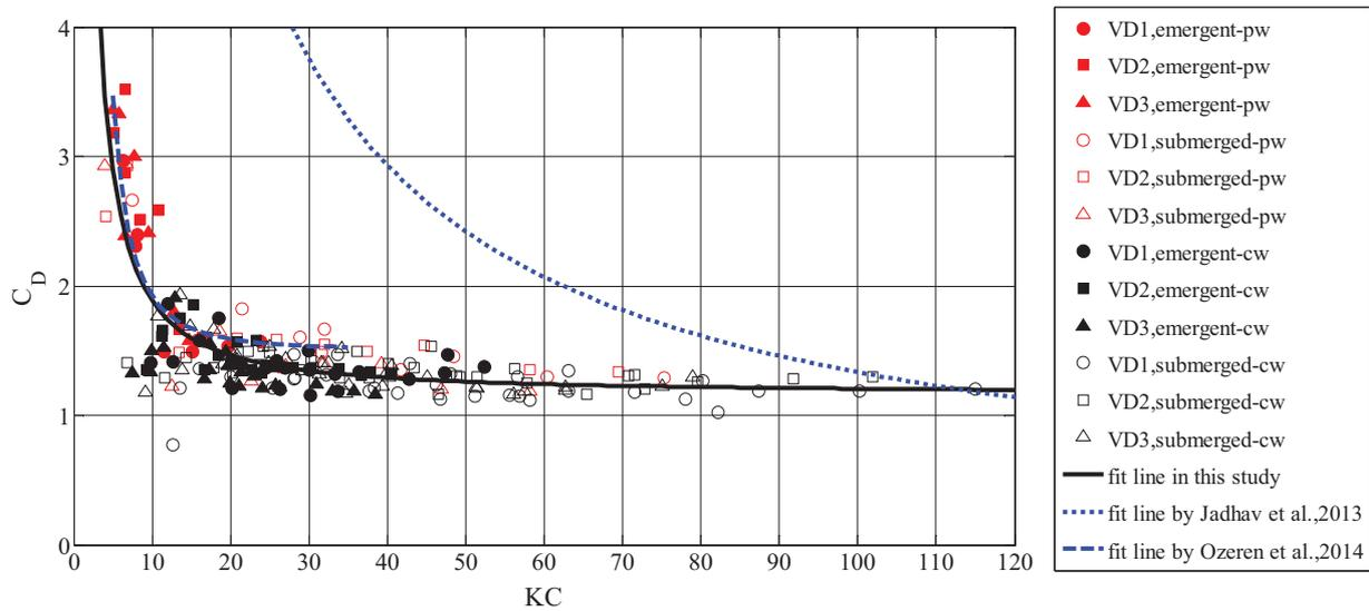
Fig. 9.  $C_D$ - $KC$  relation in both wave-only and combined wave current conditions based on direct measurement method. The red markers and “pw” stand for the results of wave-only conditions, while the black markers and “cw” stands for the results of combined wave current conditions. the fit equation from Jadhav et al. (2013) and Ozeren et al. (2014), see Table 1.
