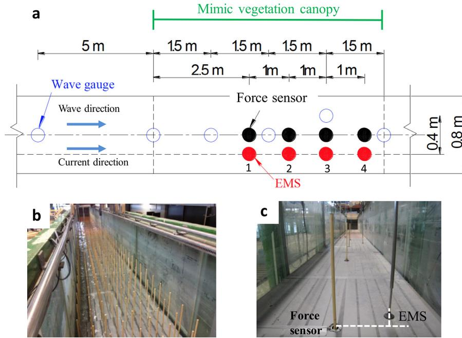
Fig. 2. Experiment set-up of Hu et al. (2014) to measure synchronized flow velocity ( $U_{wc}$ ) and acting force ( $F$ ) on wooden cylinders (mimic vegetation) at locations 1–4. (a) is the top view of the instruments and the mimic vegetation deployment. (b) is a photo of the constructed the mimic vegetation. (c) is a photo of synchronized force and velocity measurement to obtain in-phase data. The white dash lines indicate two instruments are placed at the same cross-section.
