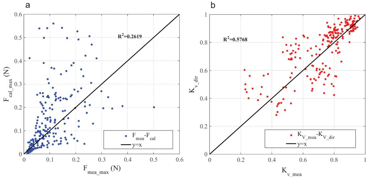
Fig. 11. (a) comparing reproduced maximum total force based on  $C_{D,cal}$  (i.e.  $F_{cal,max}$ ) with measured maximum total force ( $F_{mea,max}$ ), (b) comparing the reproduced relative wave height based on  $C_{D,dir}$  (i.e.  $K_{v,dir}$ ) with the measured relative wave height ( $K_{v,mea}$ ). The  $y=x$  lines are plotted for reference.
