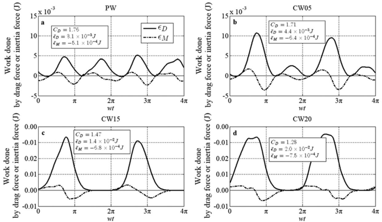
Fig. 5. Work done by acting drag force ( $\epsilon_D$ ) and inertia force ( $\epsilon_M$ ) in different hydrodynamic conditions; PW represents wave-only condition and C05W, C15W and C20W represent the wave with underlying current 0.05 m/s, 0.15 m/s and 0.20 m/s respectively.
