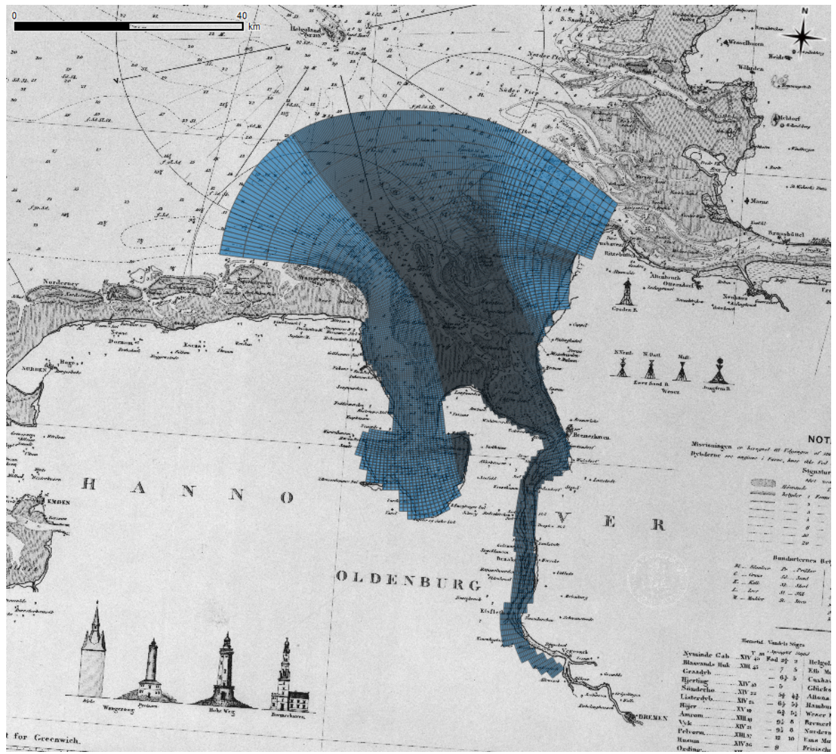
Figure 4.3: The modeling grid - model domain with a map of 1862 in the background
