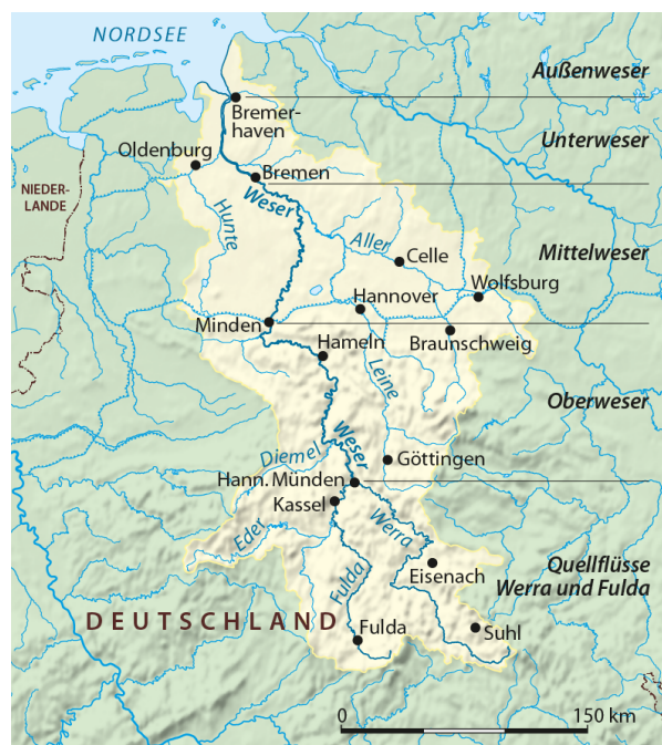
Figure 1.1: Spatial definition of the sectional separation of the Weser. Hereby, the German names translated are: Oberweser = Upper Weser, Mittelweser = Middle Weser, Unterweser = Lower Weser and Außenweser = Outer Weser
