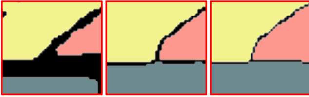
Figure 4: Stroke and uncolored pixels shown in black (left), bounded by different colored regions are retained and medially thinned (middle), and further turned into skeletal chains of pixels, suitable for vectorization (right).
