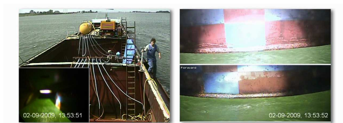
Fig.1: MS Kraichgau , experimental air supply system (left) and view inside an air cavity (right and close up left), courtesy of Damen (PELS 2 project)
