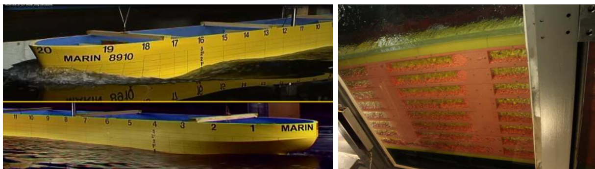
Fig.8: Model of MV Kraichgau (left) and a sample of tested bottom configuration (right)
