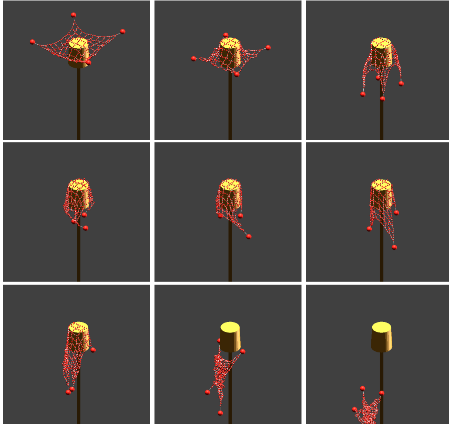
Figure 9-3: Net simulation where the net ‘rolls’ of the target.
