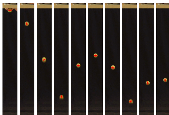
Figure A-4: Tracking of one of the experiments. The red asterisk indicates the tracked location of the tennis ball.
