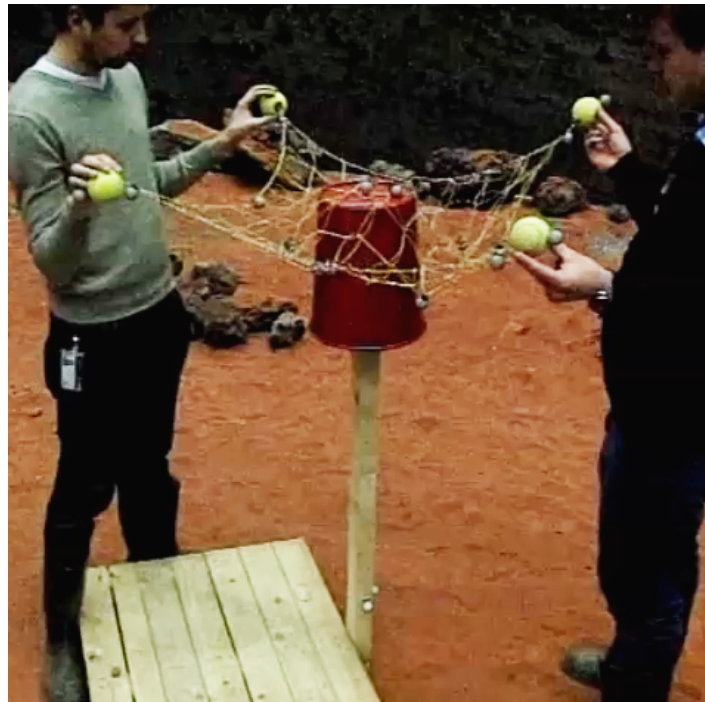
Figure 9-2: Net experiment, right before the net was dropped. Note that in this picture the Vicon markers are in fact attached to the net (silver balls).
