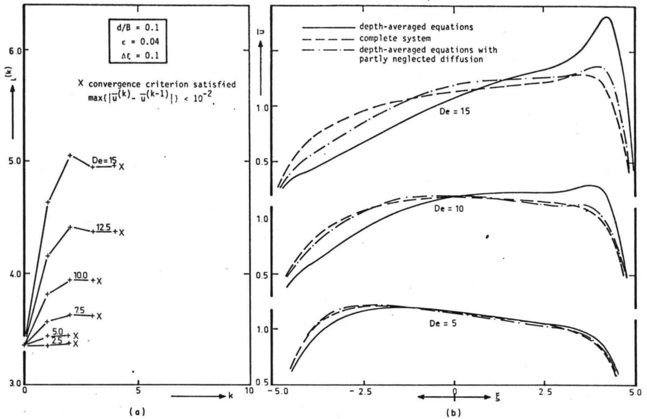
Figure 29. Solution of  $\bar{u}$  from depth-averaged equations derived from the low Dean number expansion (zero order approximation of the secondary flow)
