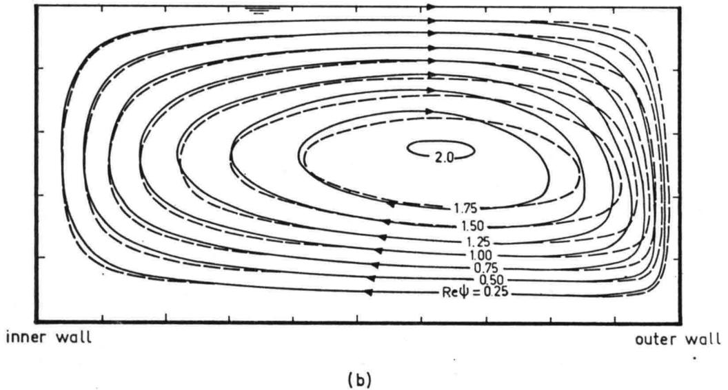
Figure 24. Influence of secondary flow inertia on the flow in a shallow channel
