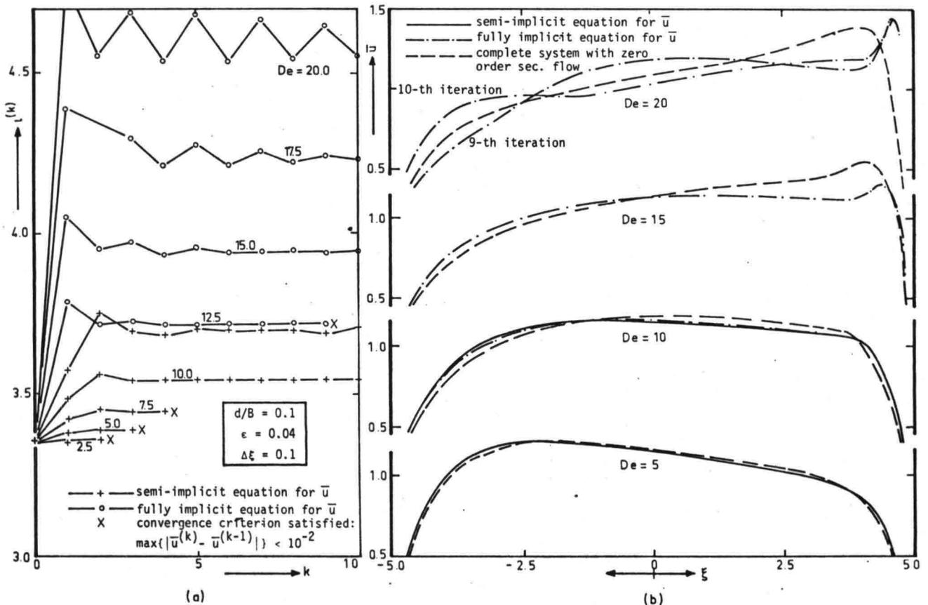
Figure 30. Solution of the depth-averaged equations derived from the low Dean number expansion (secondary flow updated in each iteration step)
