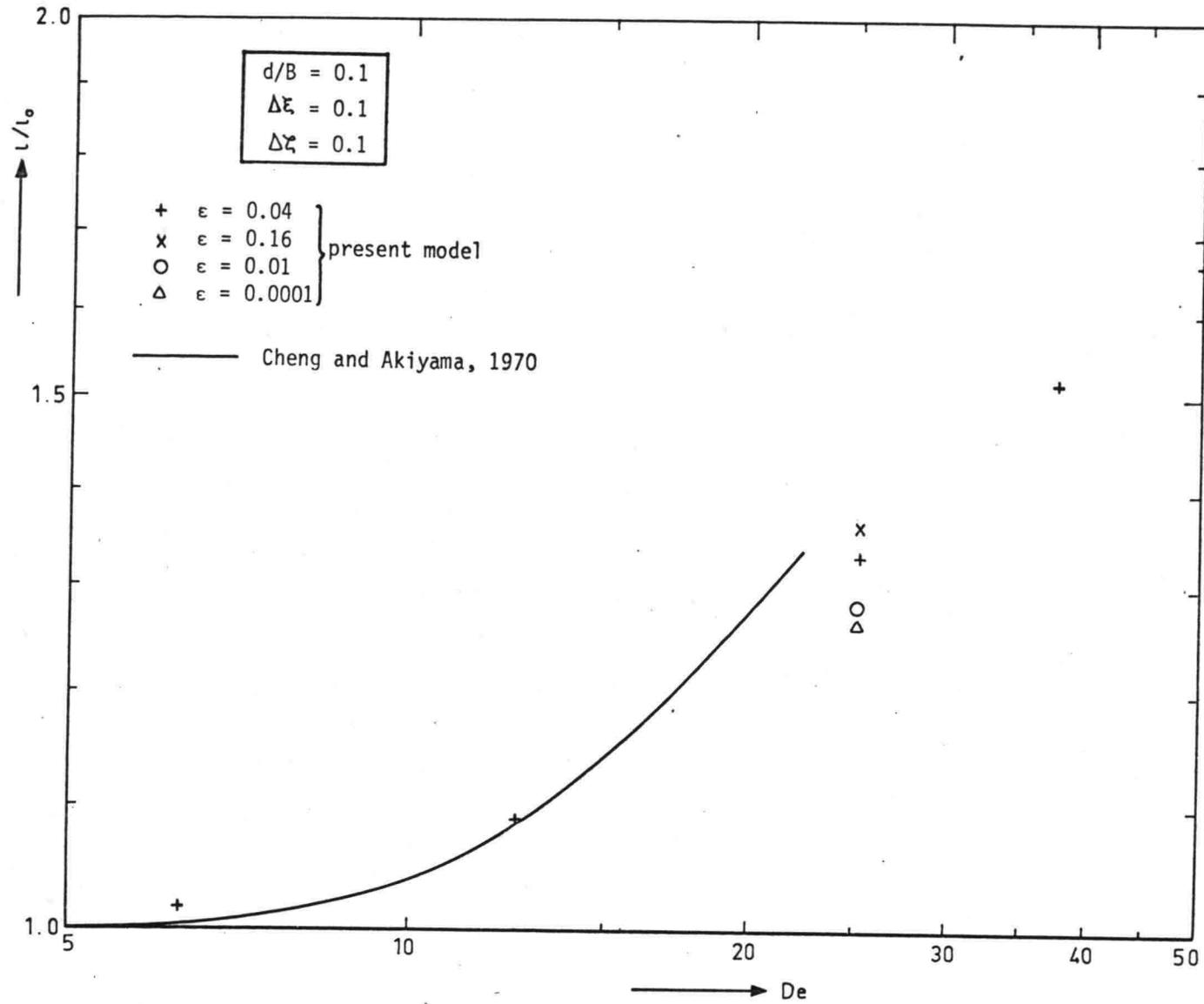
Figure 12. Influence of the Dean number on the longitudinal slope factor in a shallow channel
