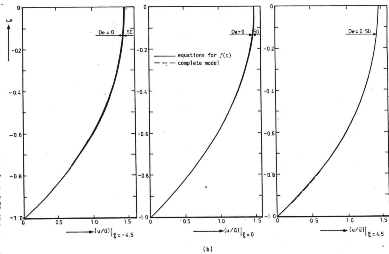
Figure 21. Separate computation of the vertical distribution of the main velocity
