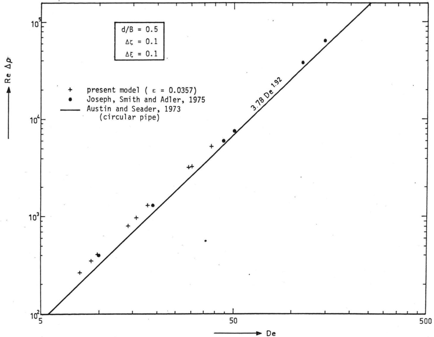
Figure 9. Transverse pressure drop at the surface compared with results for a square and a circular pipe
