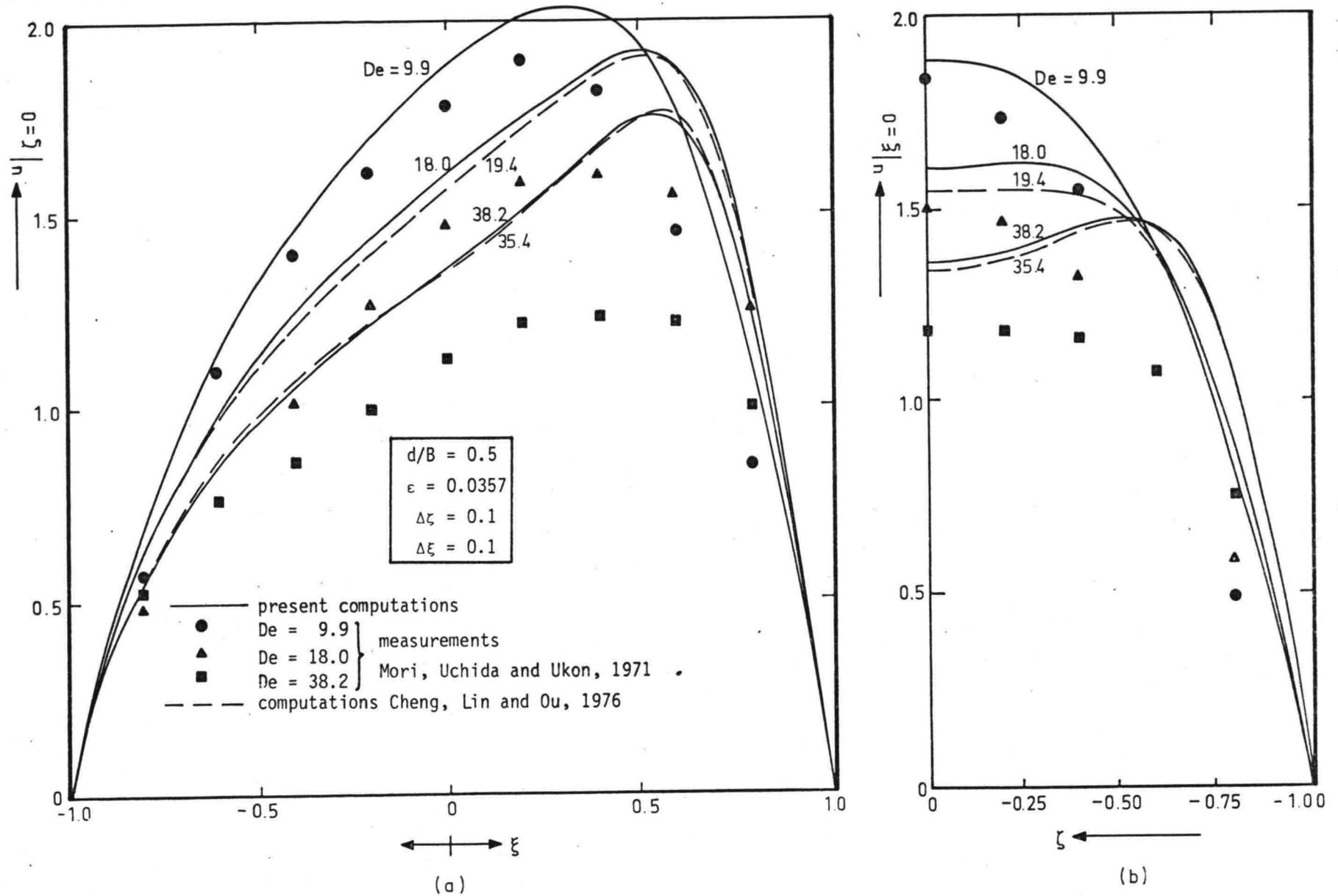
Figure 10. Comparison with Mori, Uchida and Ukon's measured data for a square pipe
