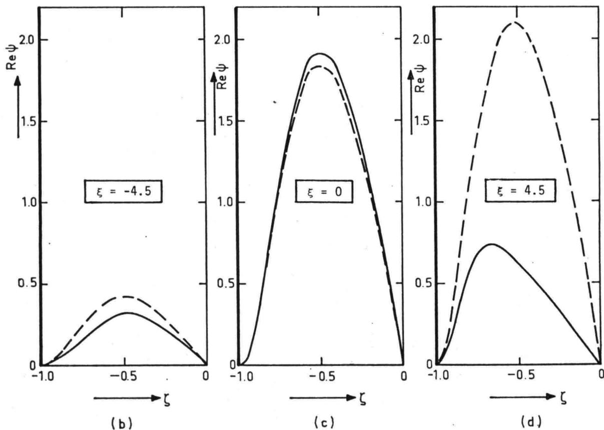
Figure 25. Influence of neglecting all radial derivatives in the stream function equation in case of a given main velocity distribution
