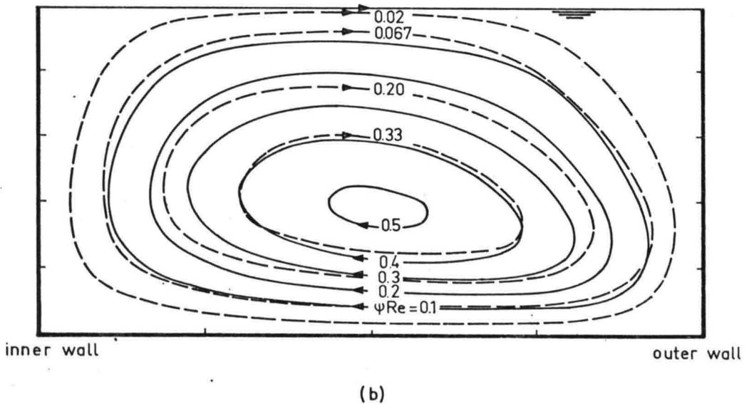
Figure 7. Transition to double helical flow pattern in a square pipe
