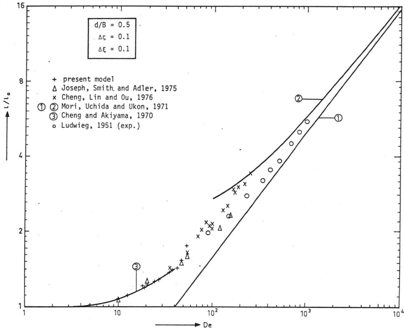
Figure 6. Longitudinal slope factor vs. Dean number for a square pipe
