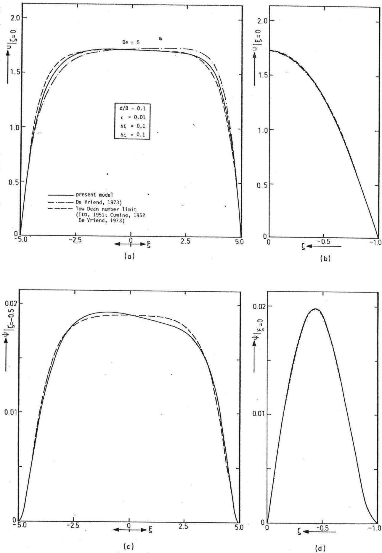
Figure 4. Comparison with analytical results for a shallow pipe at low Dean numbers
