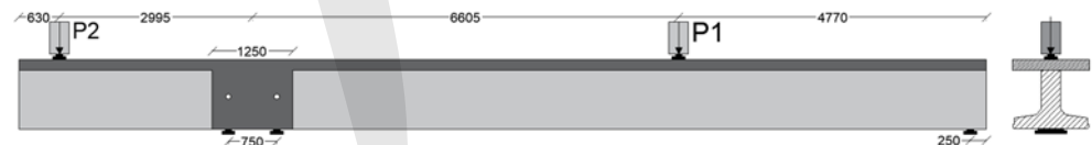
Fig. 1 Geometry of specimens and location of loading points P1 and P2 (dimensions in mm).
