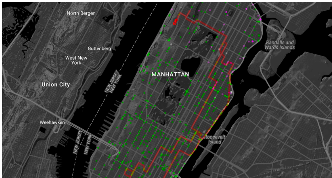
Figure 3-1: A snapshot of the simulator. Green dots represent vehicles that either have passengers on board or are on their way to pick up passengers. Pink dots represent vehicles that are driving towards areas of expected demand with no passengers on board. Grey dots represent vehicles that are idle. The snapshot furthermore shows the location and history of one of the vehicles in the fleet (represented by the red car).
