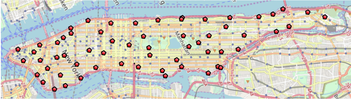
Figure 4-2: The computed location of region centres in Manhattan using the algorithm presented in Section 4-3 for a maximum reachability time t_{max} = 150 seconds.
