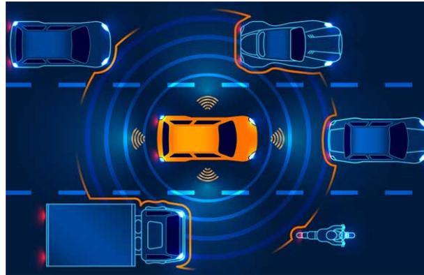
Figure 2.5: Intelligent vehicles which uses active sensing with radar to perceive the nearby traffic. Source: [59]
