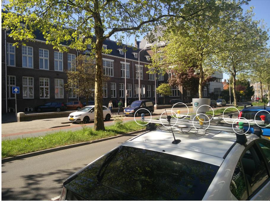
Figure 4.4: Recording one of the idle scenarios of the DriveSound. Eight microphones (white circles) are mounted on the roof of the vehicle along with a Velodyne lidar scanner, used to determine the ground truths.
