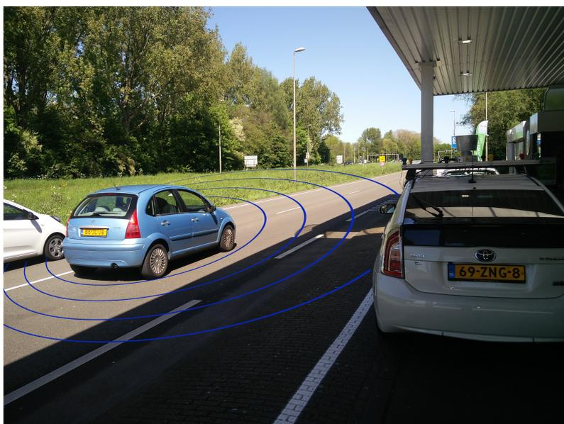
Figure 1.3: A car driving past the white listener vehicle. The sound emission from the blue target vehicle is captured by the microphones mounted on the listener vehicle.
