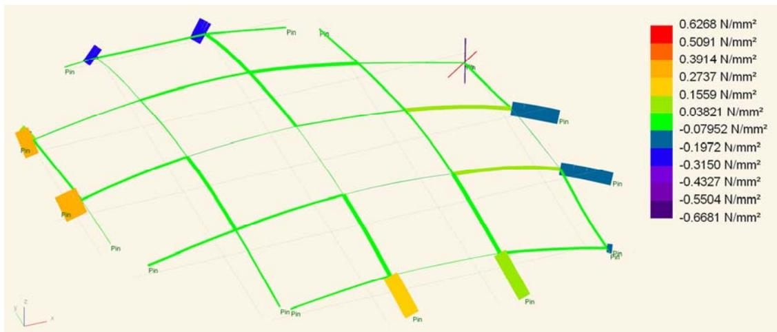
Figure 7.90: Shear stress in the elements' z-direction,  $\tau_{xz}$
