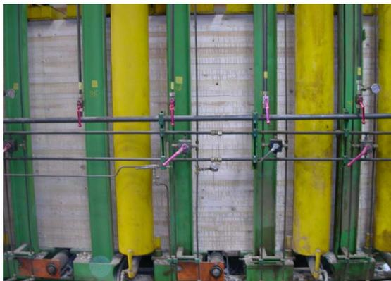
Figure 2.49: Straight laminated beam in press.
