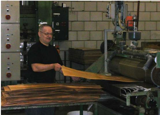
Figure 2.53: Glue is applied on laminates
