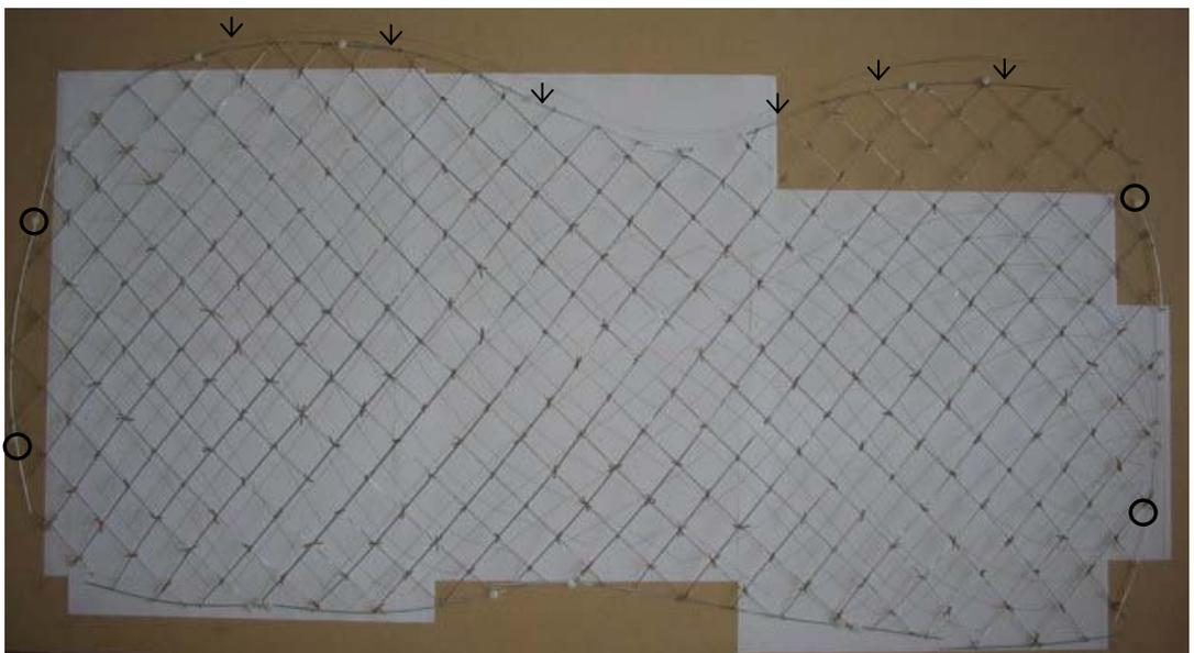
Figure A.27: The structure is tensioned by pushing on the long edge and preventing movement at the short edges.
