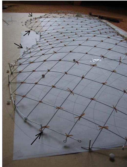
Figure A.29: By pushing from the sides, domes are shaped.
