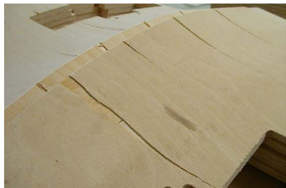
Figure 2.57: Cracks in upper layer.
