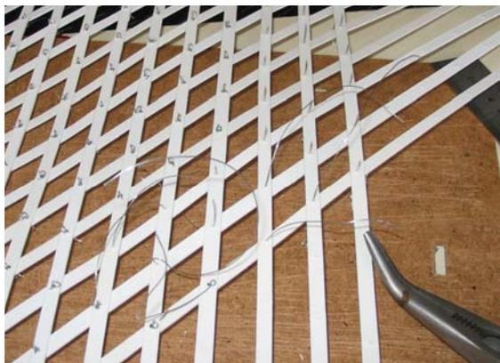
Figure A.46: The grid is tied with binding wire
