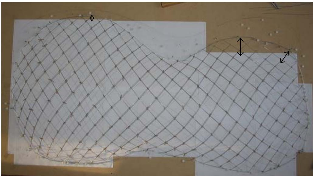
Figure A.34: Shallow dome (left) formation is almost finished. The formation of the stronger curved dome (right) needs to move upward to reach the desired height.
