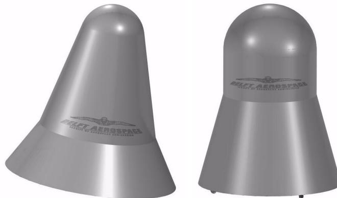
Figure 5-1: early shapes of DART vehicle with 0.25m and 0.39m nose radius, 1.3m base radius and 1.6m length
