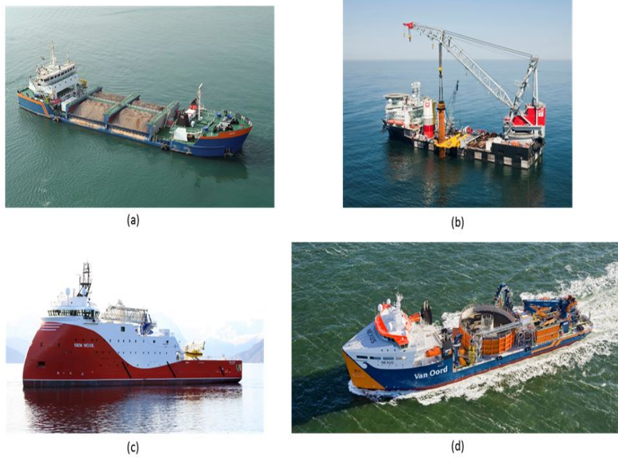
Figure A.5: (a) Rock dumping vessel,(b) Heavy lift vessel,(c) Multi-purpose vessel,(d) Cable lay vessel
