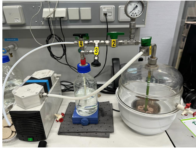
Figure 3.2: Machine used to saturate the sample with the brine solution in vacuum
