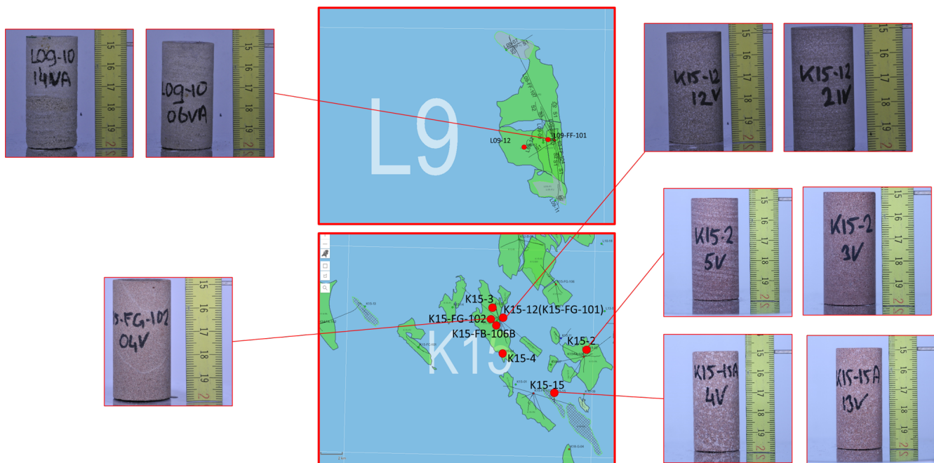
Figure 3.3: Core samples from various wells in the AOI, maps modified from nlog.nl
