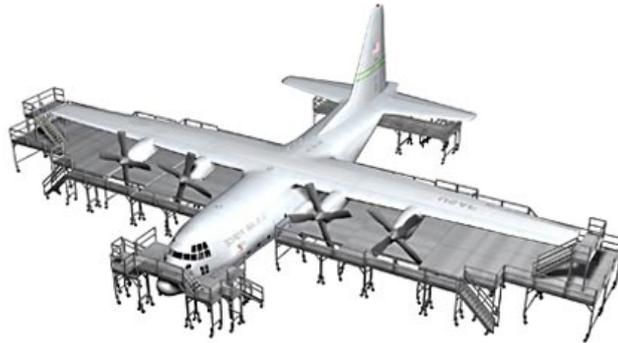
**Figure 6.15:** Lockheed C-130J Hercules maintenance platform.
