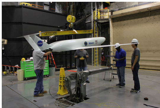
Figure 5.2: 1:11-scale D8 wind tunnel model placement
