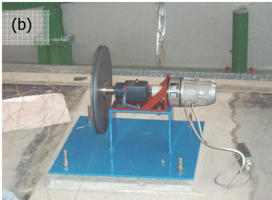
Figure 6a,b,c: Experimental set-up. a: the basin, b: the motor with the flywheel and a steel wire, c: a pulley on the other side of basin.
