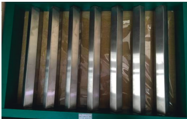
FIGURE 3: Forming mold of anti-dry-shrinkage cracking performance test specimens (mm).
