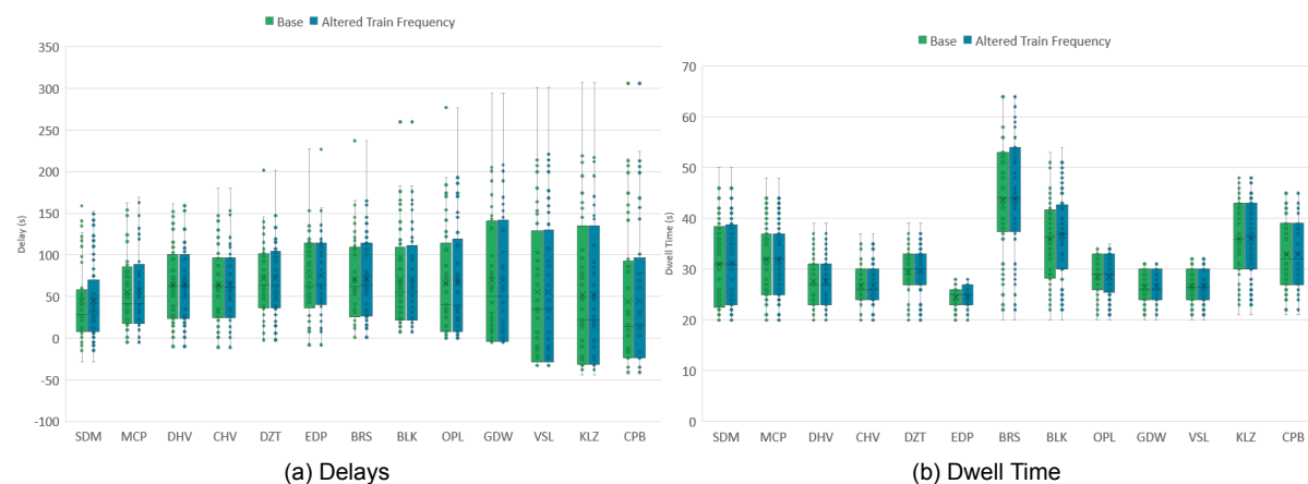
Figure 5.26: Base scenario delays and dwell times compared to the altered train frequency scenario
