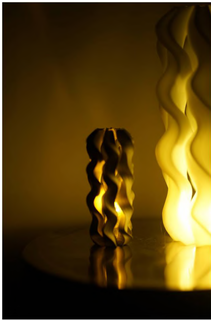
Figure 54. SLS printed lamp concepts with aluminium powder
