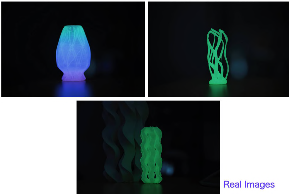
Figure 48. PLA with phosphorescent material that can glow in the dark
