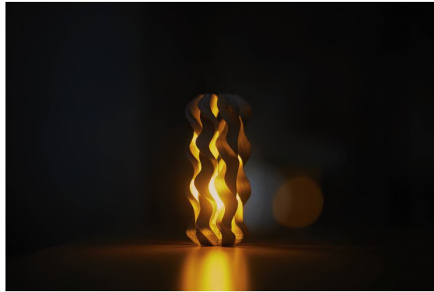
Figure 54. SLS printed lamp concepts with aluminium powder
