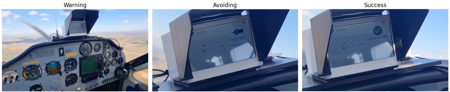
Figure 4: GA Box showing a warning sign (left), suggested speed while avoiding (middle), and successfully avoiding conflict (right). The polar plot on the left of the screen shows the relative position of the intruder.
