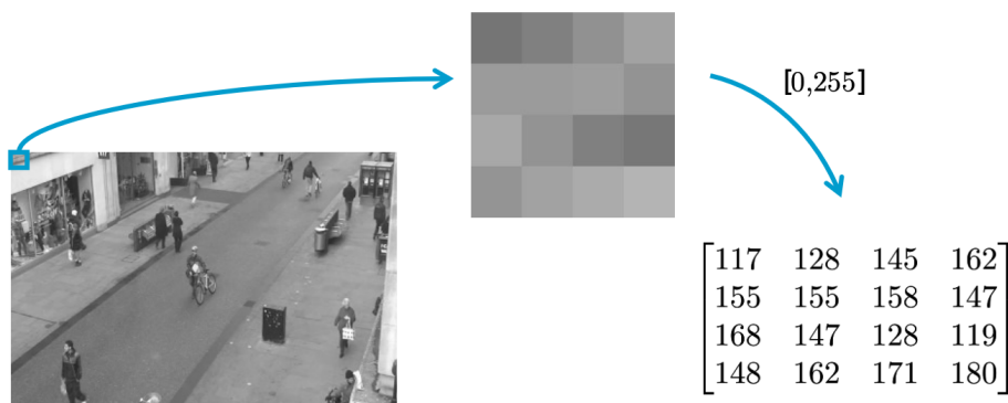
Figure 1-2: Matrix representation of (part of) a greyscale video frame [30, 4].
