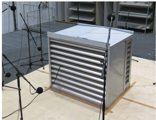
Figure 7: Measuring sound reduction in a studio (Solflex, n.d.)
