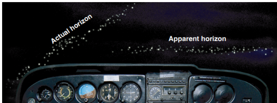
Figure 3.1: Ambient visual illusion: False horizon, happening at night. From Pilot's Handbook of Aeronautical Knowledge , by Federal Aviation Administration, 2016 [22].
