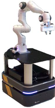
Figure 1.1: This figure presents the mobile manipulator robot from the AI for Retail (AIR) Lab Delft [1], which consists of a moving base and an arm on top. This robot consists of 10 degrees of freedom (DOF): 3 of the base and 7 of the arm.
