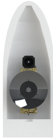
Figure 13.3: Preliminary S/C structure fitting inside the payload fairing.
