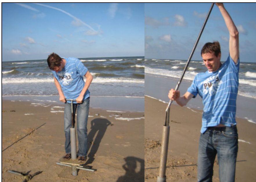
Figure D4: Operation of a pulse drill
