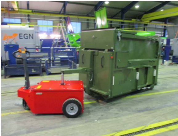
(a) Mover system for transporting press containers to pick-up point.
