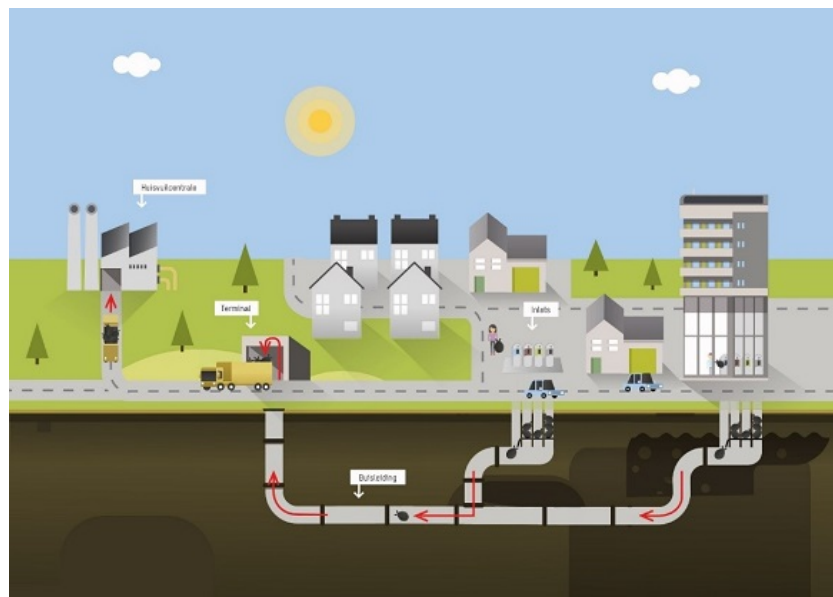
Figure 3.8: Underground Waste Transport System (OAT) [Sweco Nederland, nd]
