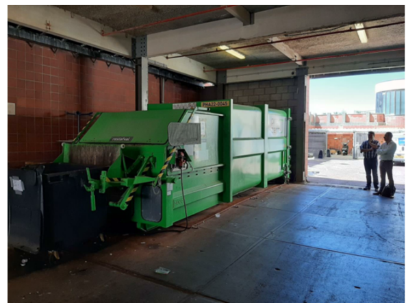
(b) Press container with tilting installation.
