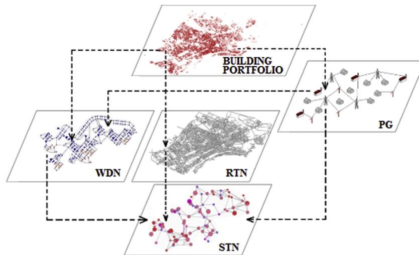
Fig. 1. Hybrid multi-layered model and interdependencies (dashed arrows).
