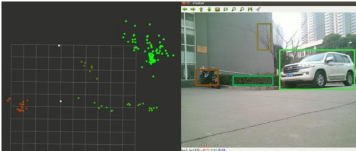
Figure 2.6: Illustration of radar scan information compared to the same scene perceived by a monocular camera. The colours correspond for different objects. Adopted from [56].
