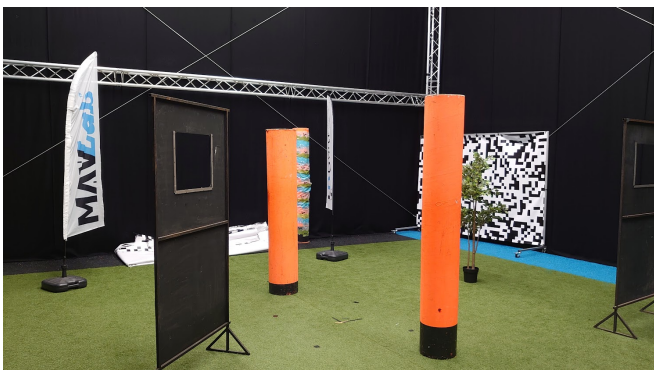
Figure 12: Image of the test setup in the CyberZoo. Notice that most objects consist of mostly vertical edges and the background has no texture.
