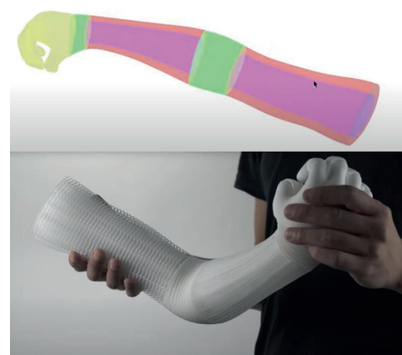
Figure 59: 3D printed arm designed by Nature Architects using function integration
