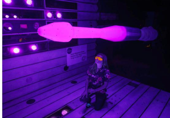
Figure 1.4: Pressure sensitive paint applied to generic launch vehicle model (source: NASA Ames Research Center)
