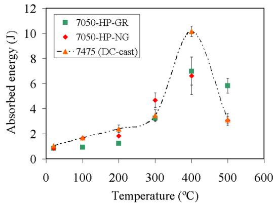
**Figure 1.** Charpy impact toughness for two 7050 alloys cast in the copper mould (GR: grain refined; NG: non-grain refined) and DC cast 7475 samples.
