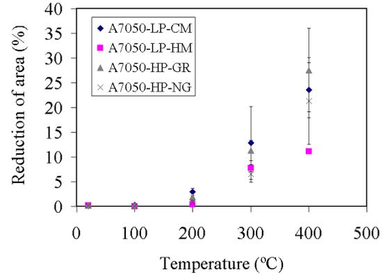
**Figure 2.** Average reduction in area of 7050 samples cast in the copper mould (see Table 1) tested at different temperatures at a strain rate of  $10^{-2} \text{ s}^{-1}$ .
