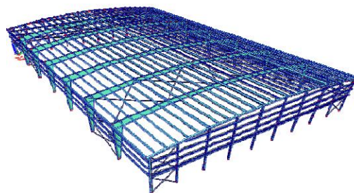
Figuur 41: Pre-engineered building (Rammant, 2009)
