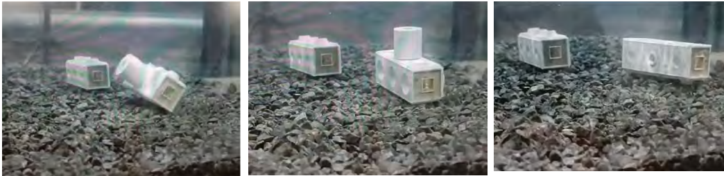
Figure 59: Result orientation perpendicular to wave current direction (in the figure from left to right)
