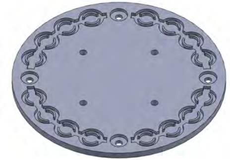
Cutouts for structural steel tubes reduces to 50mm, Saves cost and weight , creates more space for customisable tubes
