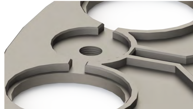
Figure 24: Sunken and tapped hole for fastening of housing 2
