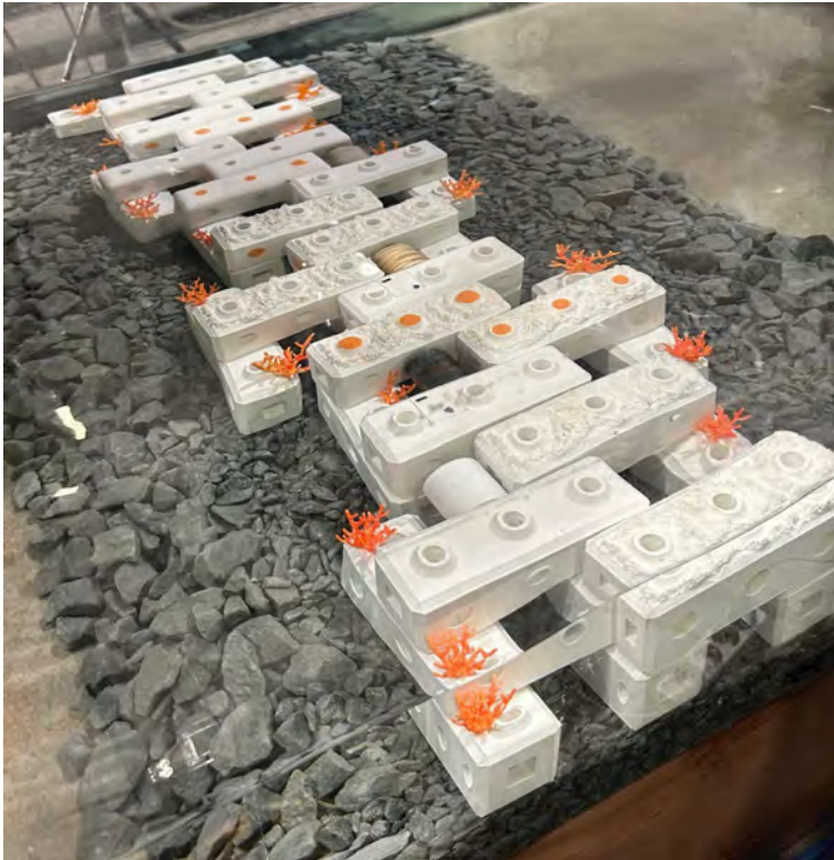
Figure 63: Four 1:20 prototypes in REB (wave current direction from left to right)
