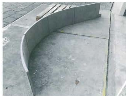
Figure 6: left: laminating of AR-glass textile as reinforcement prior to deformation of the panels; middle: curved, demoulded and aligned elements; right: 4 layers of textile visible in cut section
