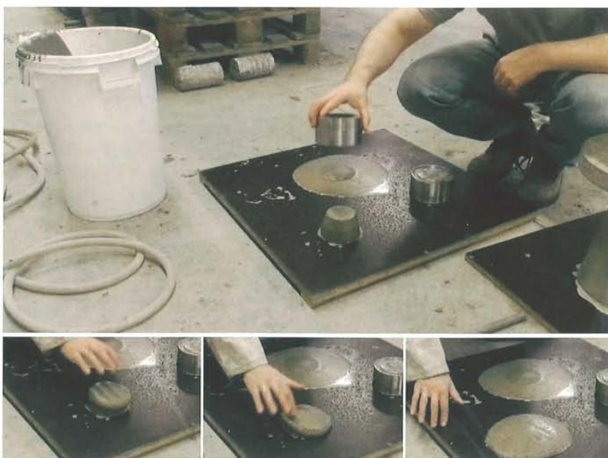
Figure 8: Slump tests on a thixotropic mixture: slight vibration by tapping the cone increases the fluidity of the fresh mixture
