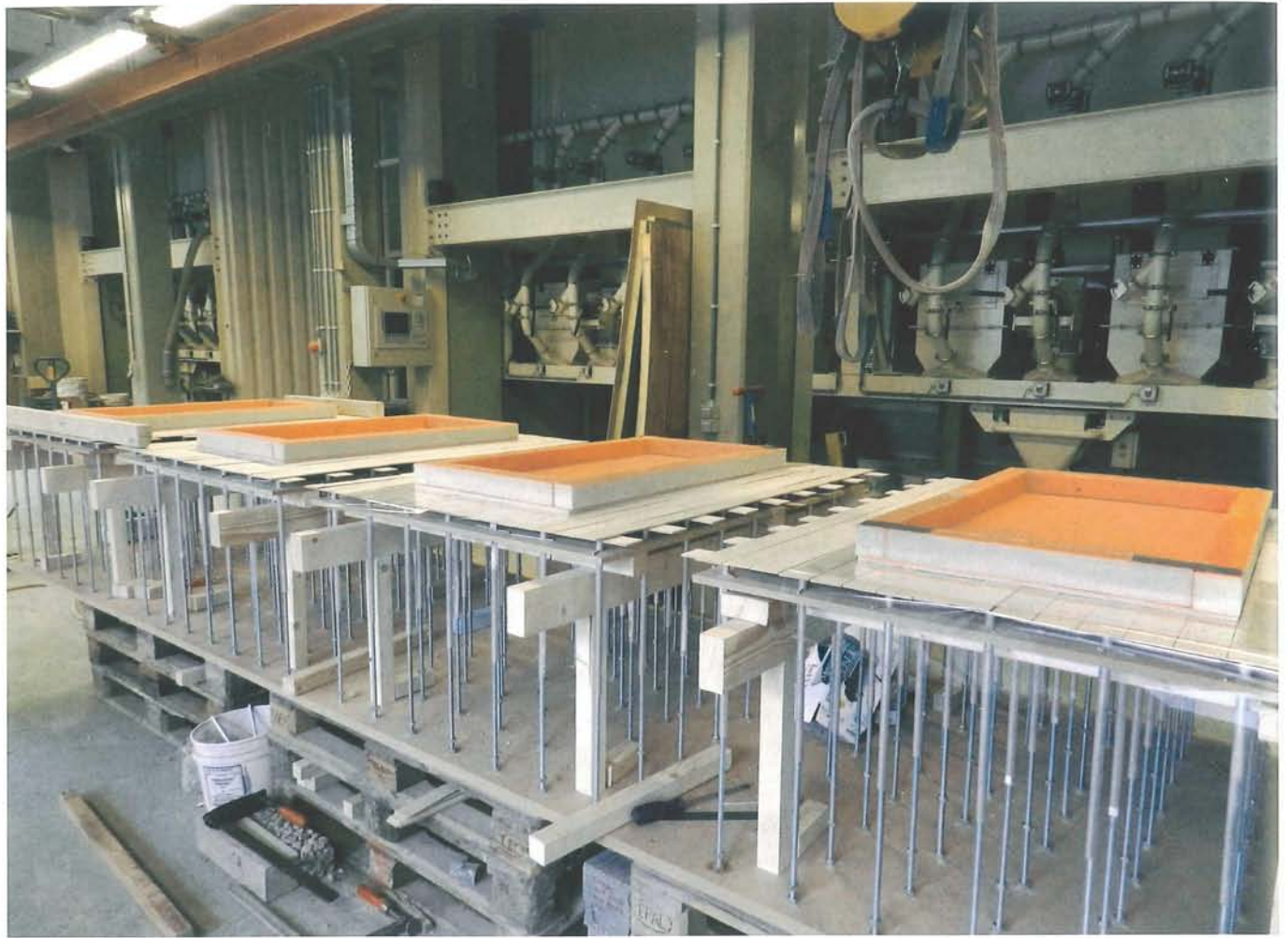
Figure 5: Test setup for parameter study in the laboratory of TU Delft (Stevin 2): four silicone moulds on a flexible base with adjustable slope and curvature. On the background the concrete mixture dosage equipment is visible.
