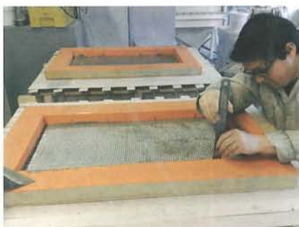
Figure 6: left: laminating of AR-glass textile as reinforcement prior to deformation of the panels; middle: curved, demoulded and aligned elements; right: 4 layers of textile visible in cut section
