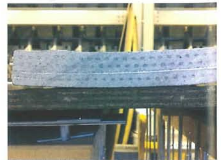
Figure 6: left: laminating of AR-glass textile as reinforcement prior to deformation of the panels; middle: curved, demoulded and aligned elements; right: 4 layers of textile visible in cut section
