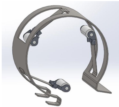
Figure 5.8: Flexure spring mechanism to prevent blossoming of a deployable stiffener. [102]
