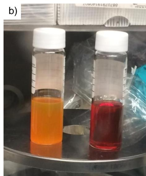
Figure 25. When washing the cores before shell synthesis, the defect emission is lowered significantly. If the cores are not washed before, the absorption (thick lines) and emission (thin lines) broaden and red-shift, as can be seen from the spectroscopic data (a) and from the sample itself (b).
