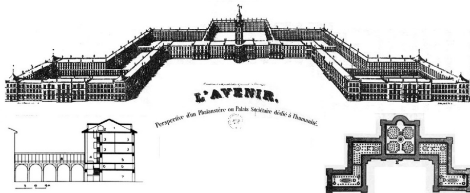
Figure 2a: The phalanstère as the future ( l'avenir ), Charles Fourier (1832). Built in the classical French palais style, the intention was for collective spaces at ground floor and second floor to be served by servant's quarters sandwiched in between. An arcaded walkway would create sheltered connection between all sections of the building.
