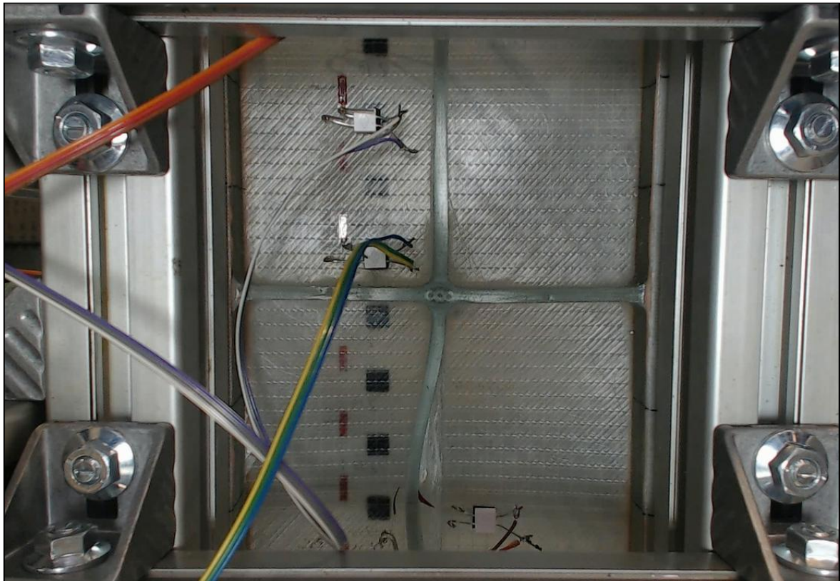
Figure 6.20: Stiffener delamination of sample orthogrid panel 2 at -110 kN
