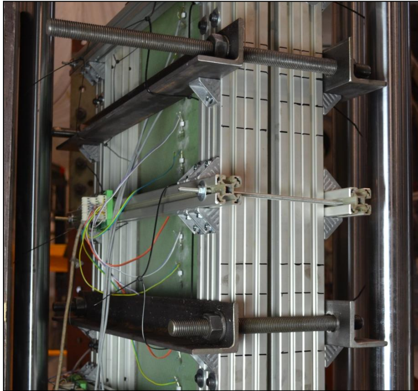
Figure 6.29: Improved aluminium frame, supported by thick steel wire
