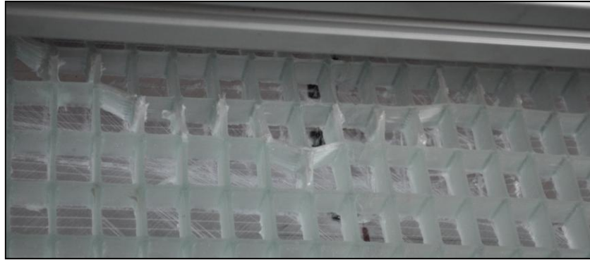
Figure 6.49: Compression failure of the grid at -163 kN (2)
