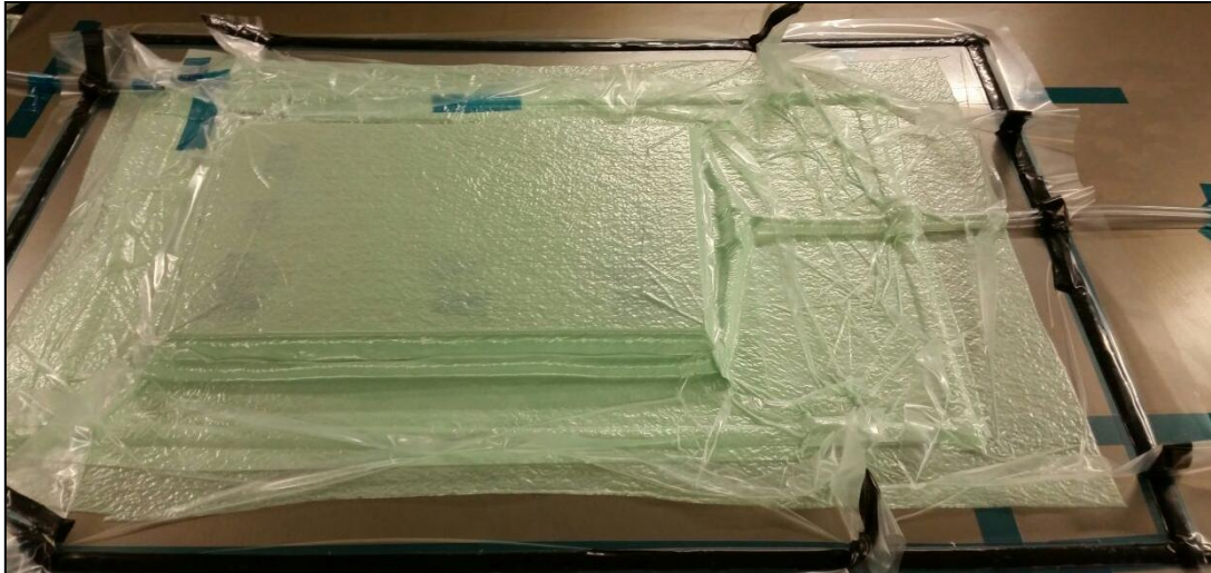
Figure 6.12: Sample orthogrid panel under vacuum
