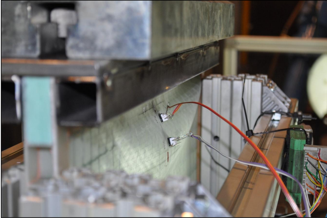
Figure 6.47: Skin delamination of the orthogrid panel at -163 kN
