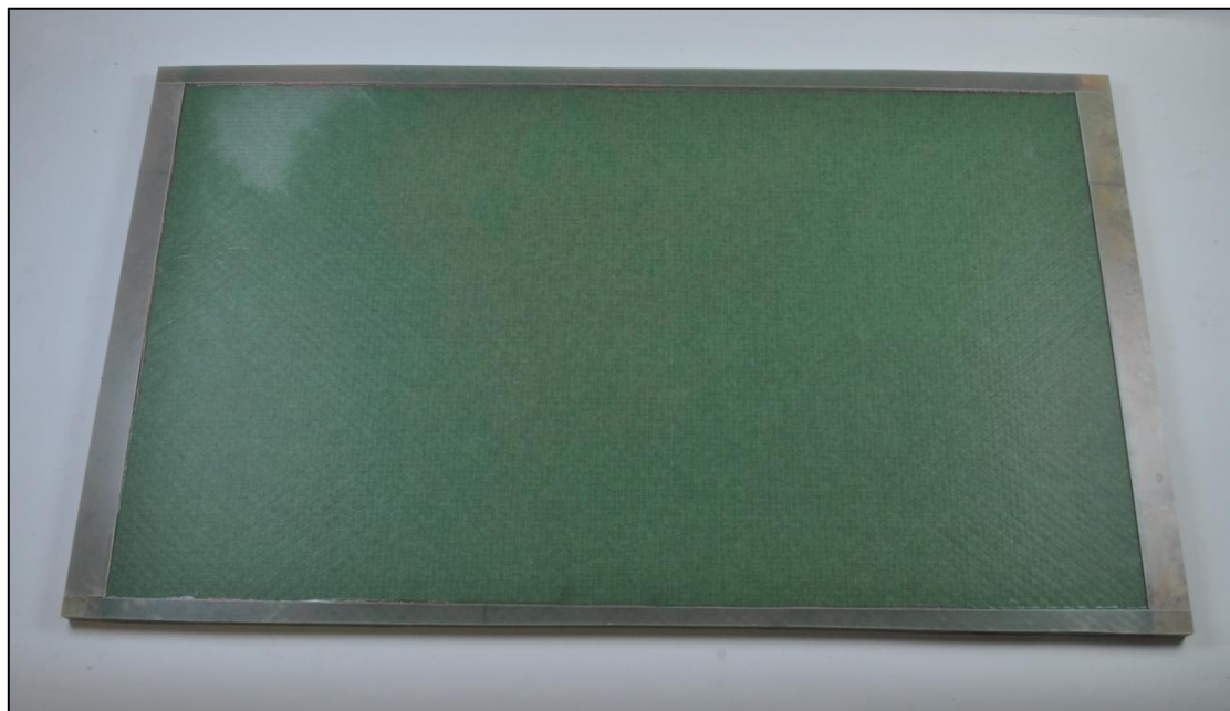
Figure 6.26: Vacuum infused sandwich panel (top)
